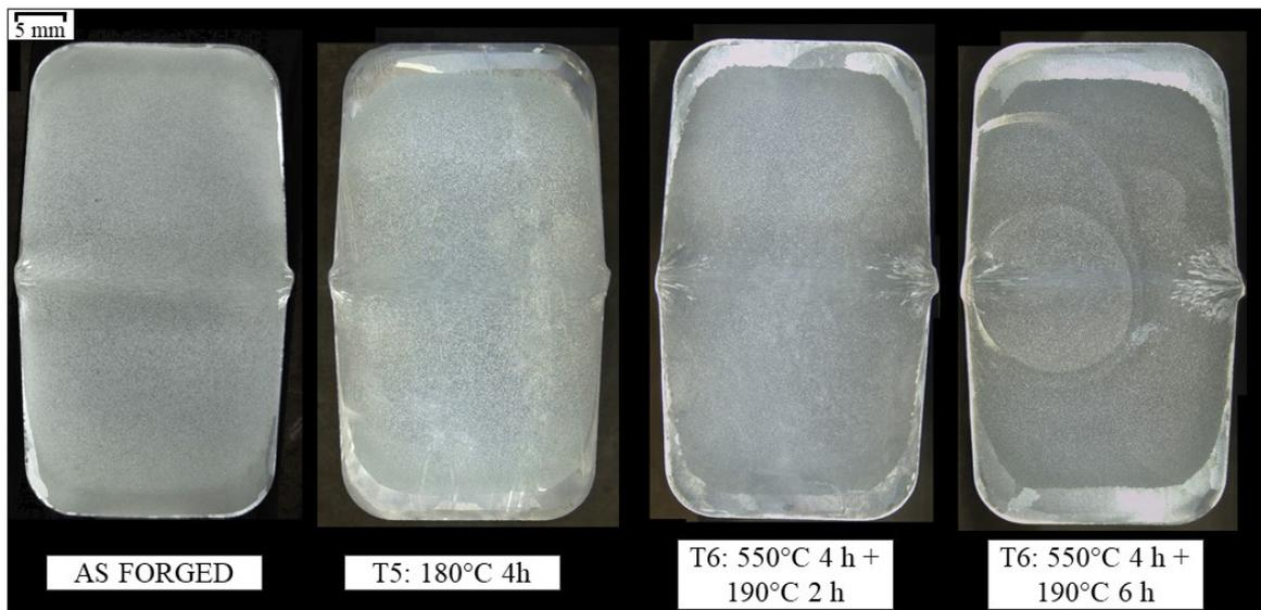
**Fig.1** - Grain structure across section of samples in the as forged and heat-treated conditions.
