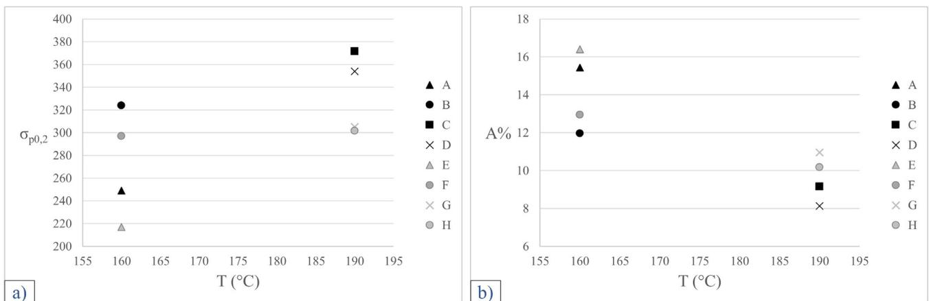
**Fig.4** - Effect of temperature on yield strength and elongation of EN AW6082 T6 Al alloy.
