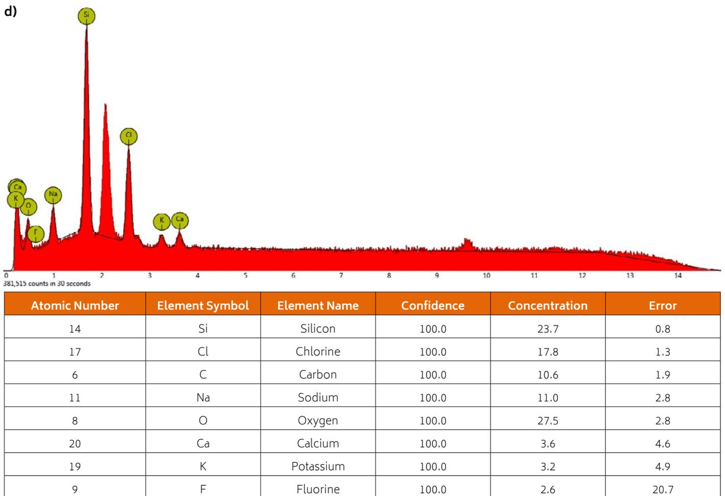
**Fig.3/6** - a, b, c and d show the graphical representation and concentration values of the elements according to the EDS results for different regions of the PLC-21 surface, respectively.
