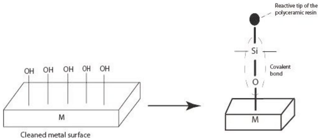
**Fig.1** - Covalent bonding with metal surface and the ceramic backbone of the polyceramic resin [26-29].
