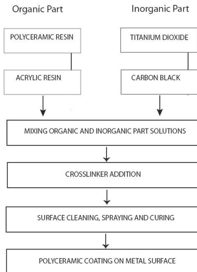
**Fig.3** - Preparation scheme for Polyceramic coating.
