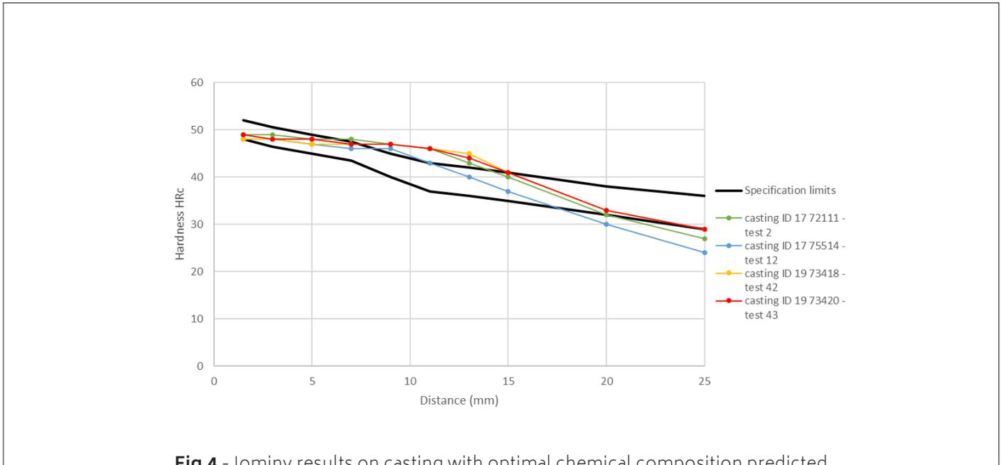
**Fig.4** - Jominy results on casting with optimal chemical composition predicted by the ANN-based predictor
