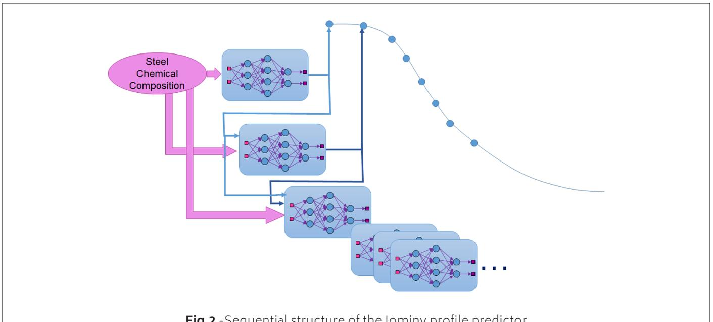
**Fig.2** -Sequential structure of the Jominy profile predictor
