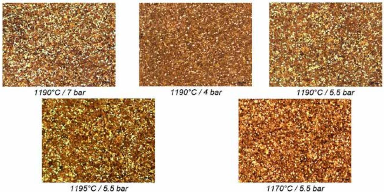
**Fig. 5** - MC90 Internet microstructures after solution annealing with different parameters and aging at 590°C.
