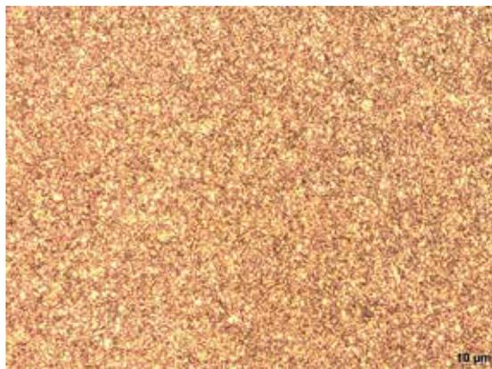
**Fig. 1** - MC 90 Intermet microstructure in longitudinal direction prior to the heat treatment (500x)
