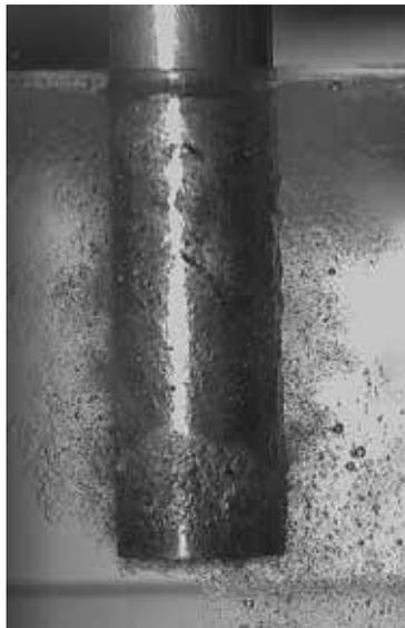
**Fig. 3 - a)** Quenching in pure water 1 second after immersion.
