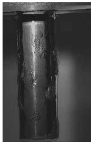
**Fig. 3 - f)** Quenching in silicate solution 3 seconds after immersion.
