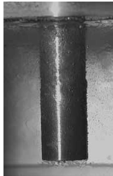
**Fig. 3 - c)** Quenching in pure water 3 seconds after immersion.
