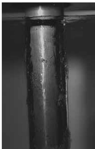
**Fig. 3 - e)** Quenching in silicate solution 1.75 seconds after immersion.
