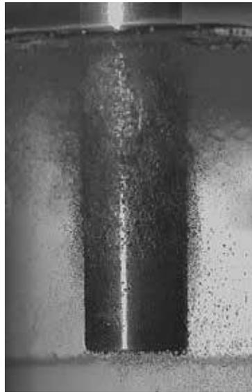
**Fig. 3 - b)** Quenching in pure water 1.75 seconds after immersion.
