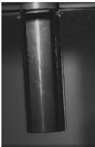
**Fig. 3 - d)** Quenching in silicate solution (35.5 wt.-%) 1 second after immersion.
