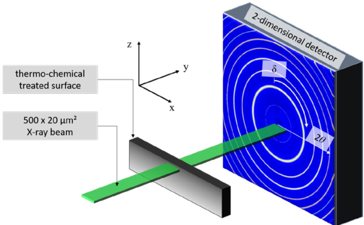
**Fig. 1** - Experimental setup of the CSmicroXRD experiment at DESY in Hamburg. The cross-section of the thermo-chemical treated sample is being scanned in transmission diffraction geometry by moving the sample in the beam along the z-axis with an increment of  $\sim 20 \mu\text{m}$ . At each scanning position, two-dimensional X-ray diffraction data are collected using a 2D detector.
