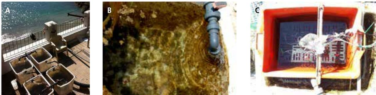
**Fig. 1** - Immersion environments: a) natural sea water, overview of the 200 L mesocosms exposed to the photoperiod; b) natural sea water, internal view of one of the 200 L mesocosms; c) artificial sea water, view of the 50 L tank containing the samples immersed in NaCl solution. This tank was partially immersed in a 200 L mesocosm which acted as thermostatic bath.
