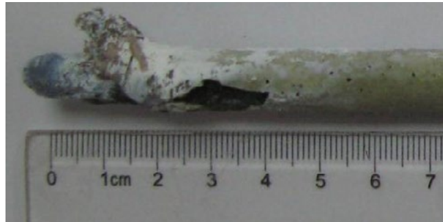
Fig. 8 – Pure calcium cored wire melting appearance
