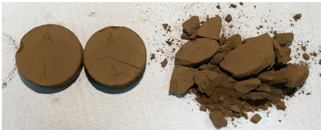
Fig. 8 – Two samples of series A (left) and of series B (right) after the drop test
