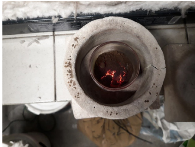
Fig. 3 – Image of the crucible insulated with alumina block.
