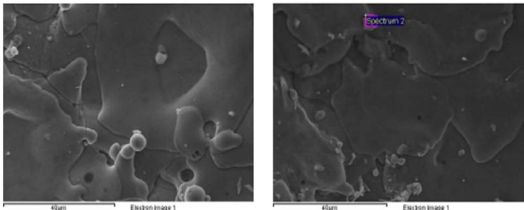
**Fig. 8** – SEM images of the micro holes on stainless steel, brass electrode, peak current and voltage (a) Low/Low (b) High/High.
