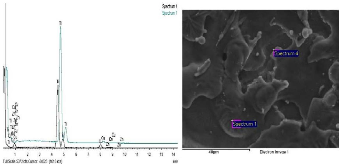
**Fig. 4** – EDX spectrum of two micro hole areas on titanium (brass electrode, peak current: high, voltage: low).
