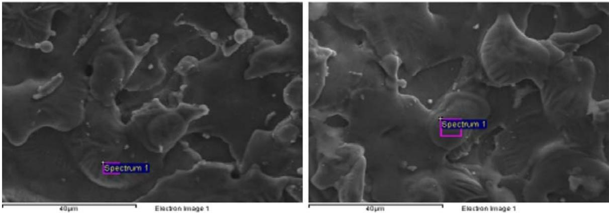
**Fig. 3** – SEM images of the micro holes on titanium, brass electrode, peak current and voltage (a) Low/Low (b) High/Low.
