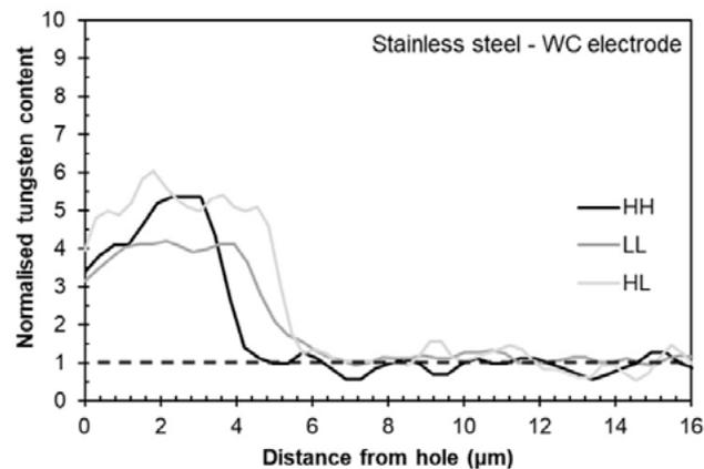
**Fig. 7** – Normalised distribution of tungsten on the stainless steel workpiece as function of the distance from the hole wall, detected by EDX, varying peak current and voltage.
