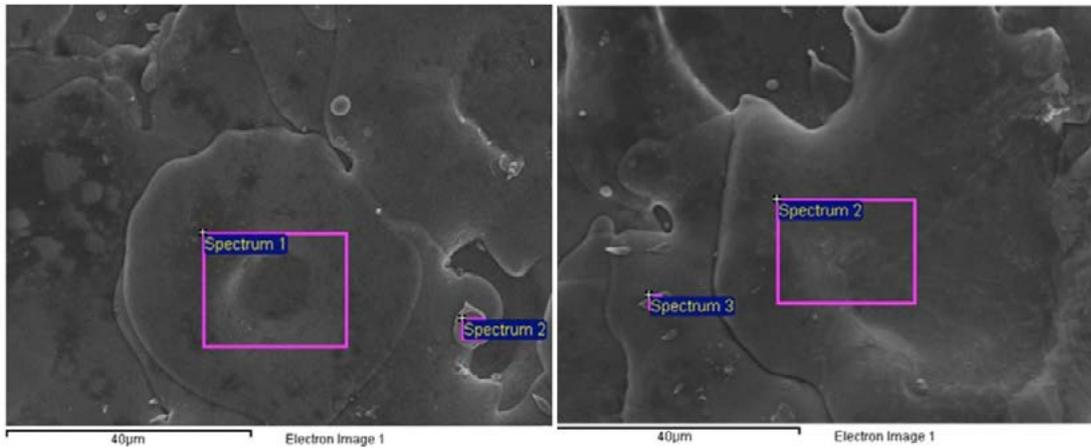
**Fig. 5** – SEM images of the micro holes on stainless steel, tungsten carbide electrode, peak current and voltage (a) Low/Low (b) High/High.
