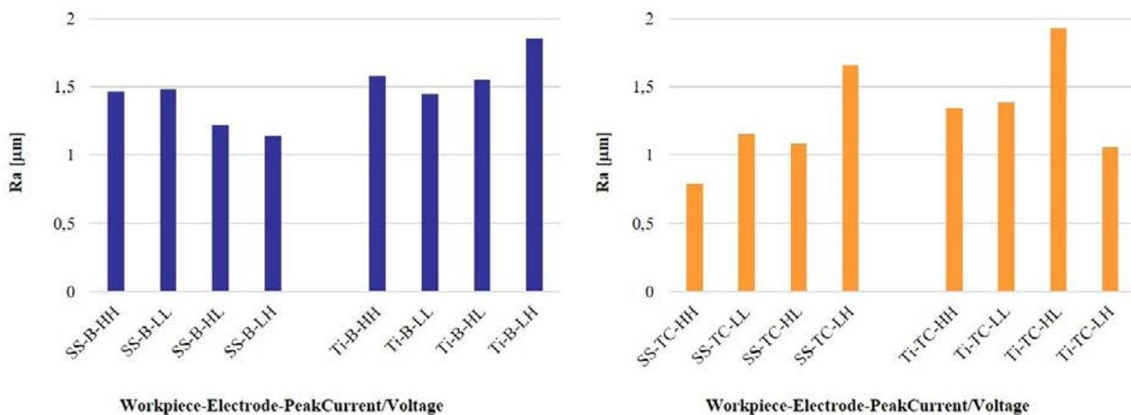
**Fig. 10** – Axial surface roughness (Ra) of holes obtained on both stainless steel (SS) and Titanium (Ti) using different process parameters combination and different electrodes.
