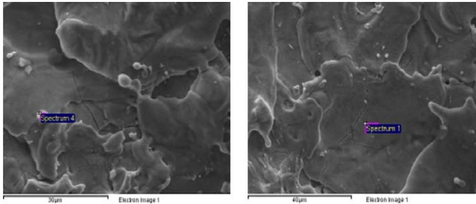
**Fig. 1** – SEM images of the micro holes on titanium, tungsten carbide electrode, peak current and voltage (a) Low/Low (b) High/Low.
