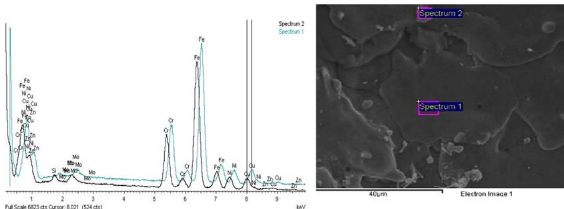
**Fig. 9** – EDX spectrum of two micro hole areas on stainless steel (brass electrode, peak current: high, voltage: high).
