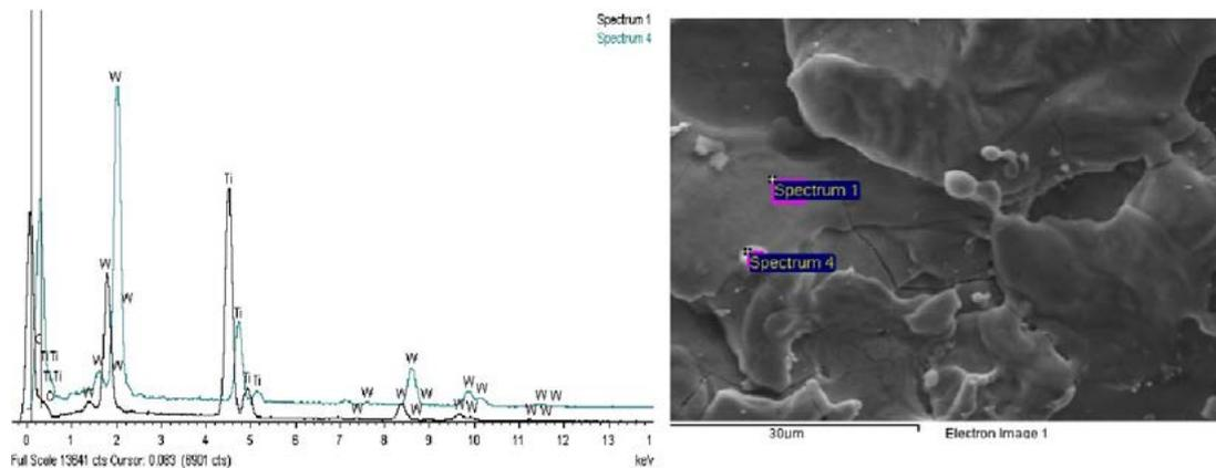
**Fig. 2** – EDX spectrum of two micro hole areas on titanium (tungsten carbide electrode, peak current: low, voltage: low).
