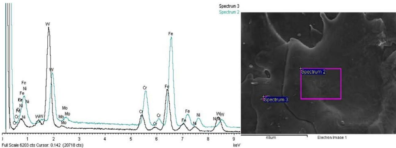
**Fig. 6** – EDX spectrum of two micro hole areas on stainless steel (tungsten carbide electrode, peak current: high, voltage: high).
