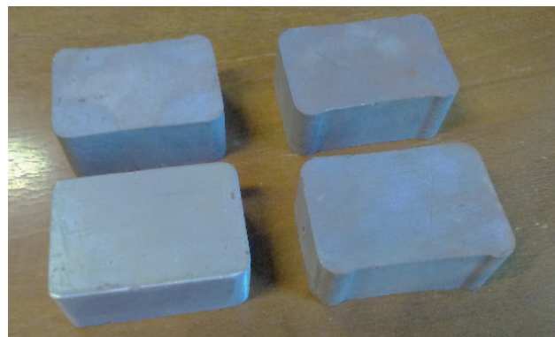
Fig. 1 – Sample size used for the heat treatment tests: 50x70x30 mm
