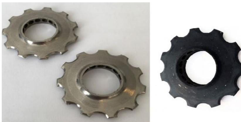
**Fig. 8** – 3D printed pulley wheels in titanium grade 5 (printed by the Danish Technological Institute, DTI). Left) Part after post finishing; Right) after surface hardening (carbo-oxidation) – cf. treatment in Fig. 9.
