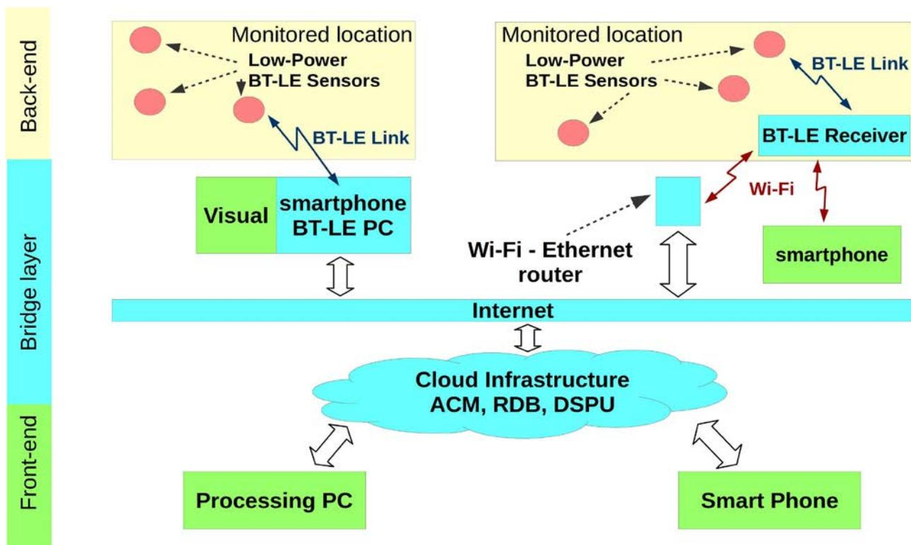
Fig. 1 – Environmental monitoring system 3 layer architecture
