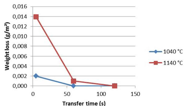
**Fig. 7** - Effect of the solution annealing temperature and quenching transfer time on the ASTM G48-A 24h / 40 °C pitting corrosion weight loss. The specimens with a weight loss were affected by pits visible at 20x magnification.
