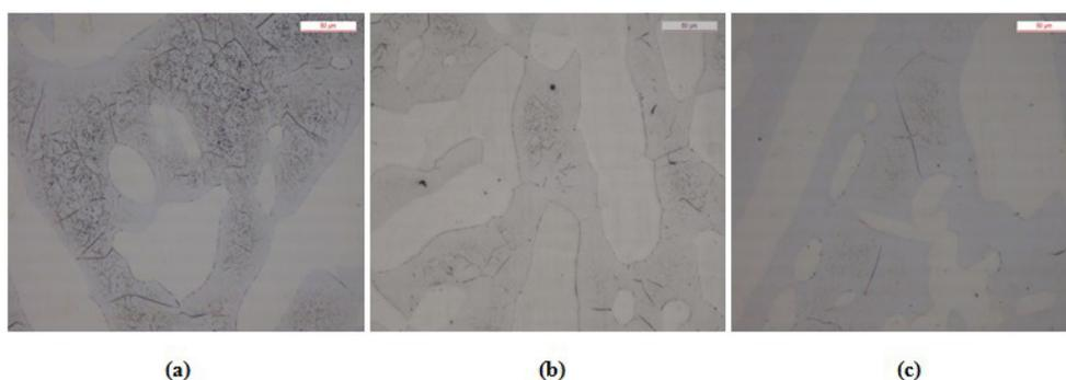
**Fig. 3** - optical micrographs of the blocks solution annealed at 1140 °C and quenched with a transfer time (a) < 5 s, (b) 60 s and (c) 120 s. The reference bar in the left top corner is for 50  $\mu\text{m}$ . Ferrite is the dark grey phase.
