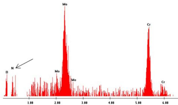
**Fig. 5** - X-EDS analysis of the precipitate highlighted by the green arrow tip in fig. 4.a
