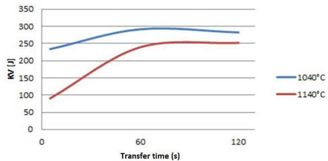
**Fig. 6** - Effect of the solution annealing temperature and quenching transfer time on the -46 °C Charpy impact test fracture energy trend (average of 3 values).
