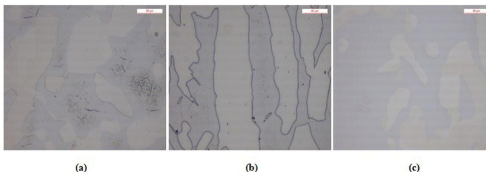
**Fig. 2** - optical micrographs of the blocks solution annealed at 1040 °C and quenched with a transfer time (a) < 5 s, (b) 60 s and (c) 120 s. The reference bar in the left bottom corner is for 50  $\mu\text{m}$ . Ferrite is the dark grey phase.
