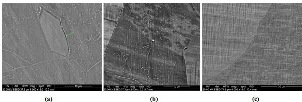
**Fig. 4** - electronic micrographs of the blocks solution annealed at 1140 °C and quenched with a transfer time (a) < 5 s, (b) 60 s and (c) 120 s. The reference bars are for (a)-(b) 10  $\mu\text{m}$  and (c) 30  $\mu\text{m}$ . Ferrite is the dark grey phase
