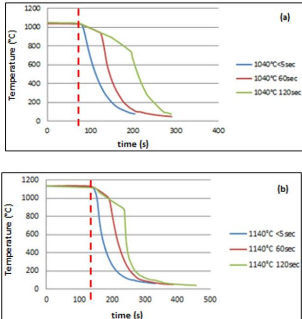
**Fig. 1** - quenching time-temperature charts of the trial blocks starting from a) 1040 °C and b) 1140 °C solution annealing temperatures. The data were collected by a contact thermocouple embedded in the block core. The red dashed lines highlights the instant of the removal from the furnace
