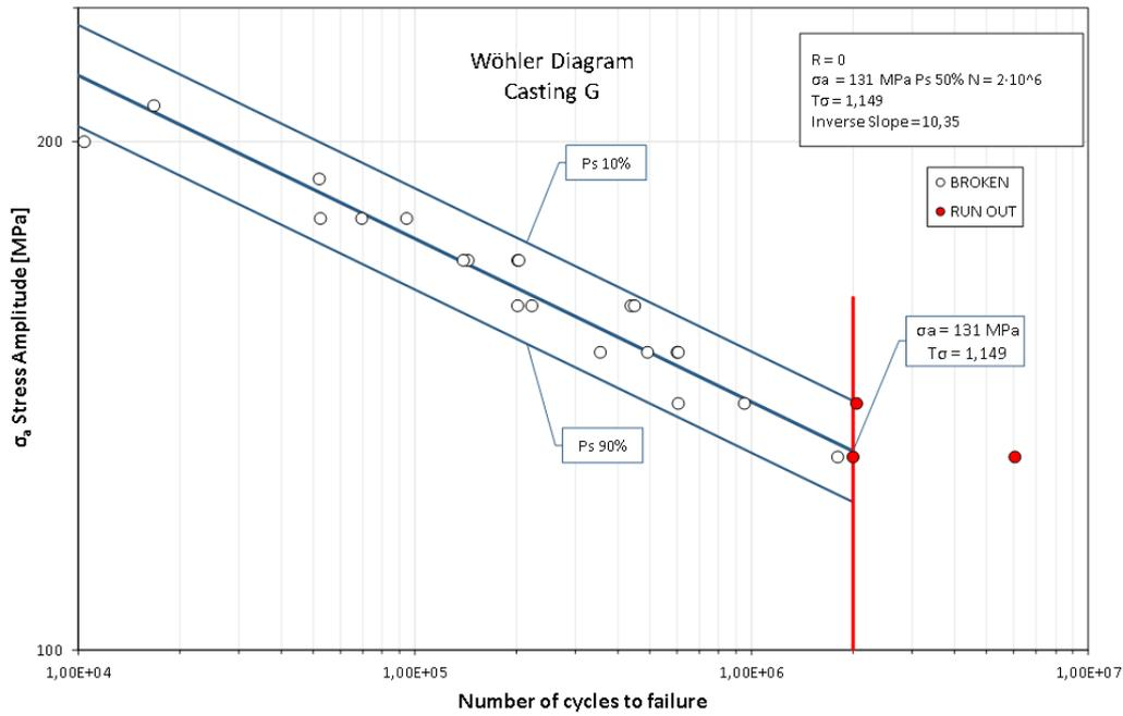
Fig. 3 - Fatigue life of specimens taken from casting G
