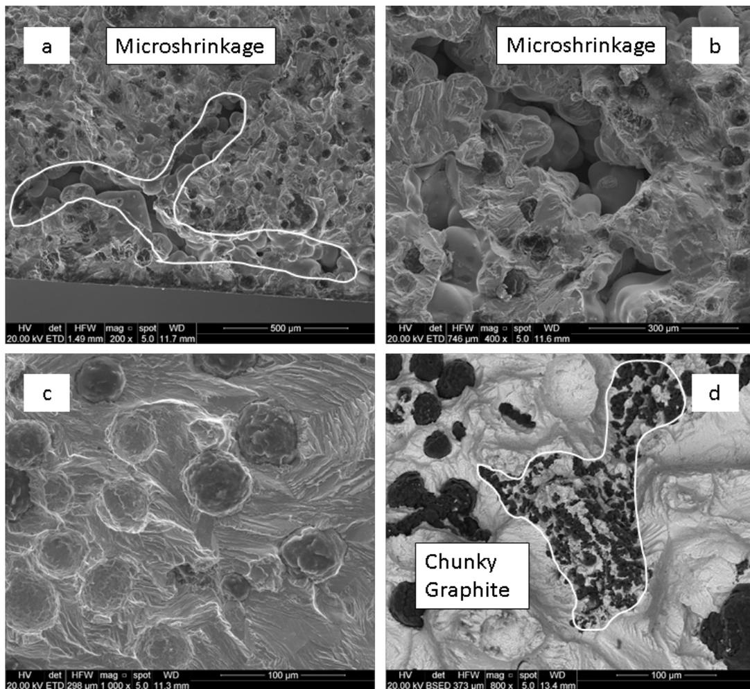
**Fig. 5** - SEM micrographs of crack initiation, showing microshrinkage porosity (a,b), propagation zones in the presence of spheroidal graphite (c) and chunky graphite (d)
