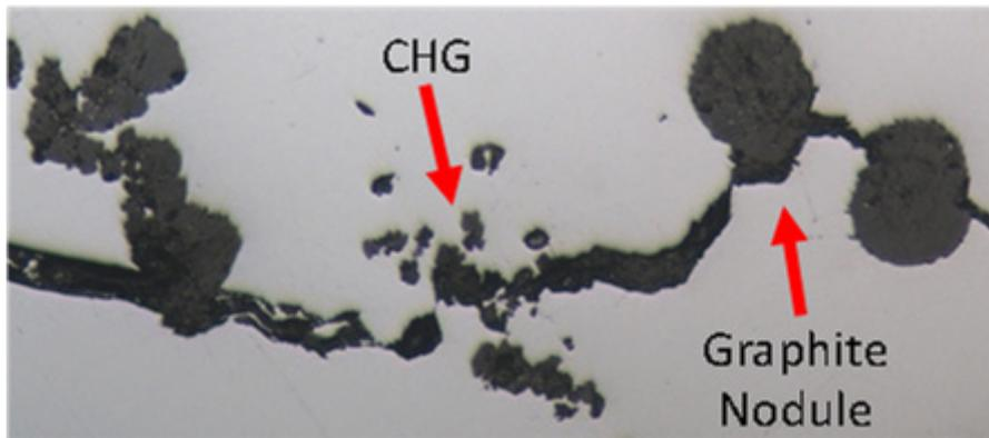
**Fig. 6** - Cross sectional view of the fracture surface showing that fatigue crack passes around the graphite nodule while propagates through the chunky graphite (CHG)
