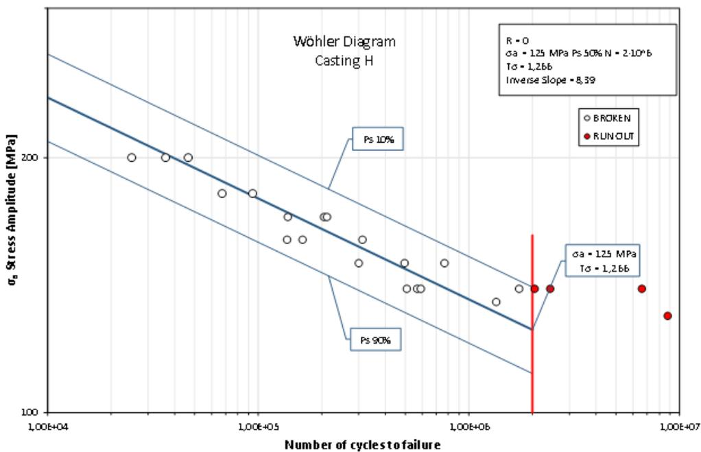
Fig. 4 - Fatigue life of specimens taken from casting H
