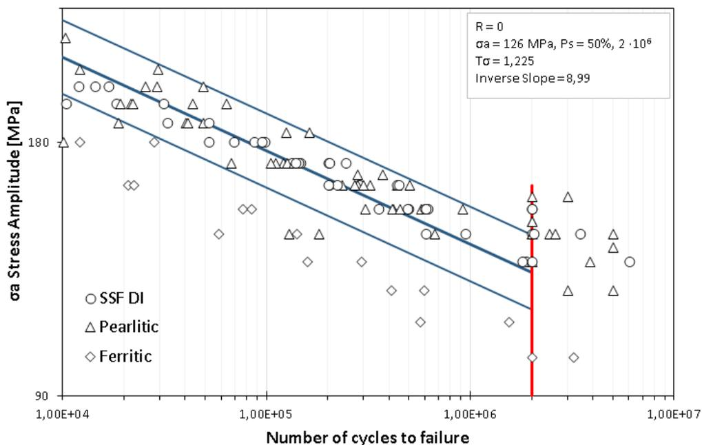
**Fig. 7** - Fatigue life of specimens taken from pearlitic, ferritic and solution strengthened ferritic heavy section ductile cast iron castings
