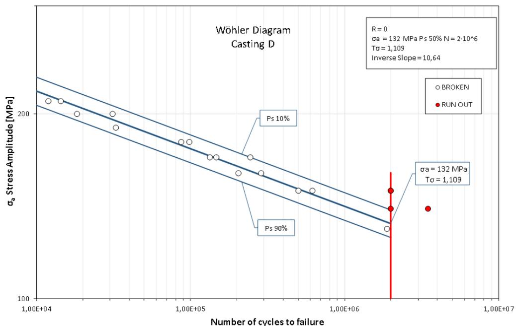
**Fig. 2** - Fatigue life of specimens taken from casting D
