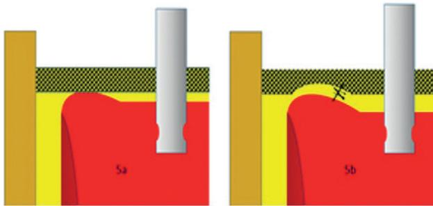
**Fig. 5** - Liquid pool thickness by application of flux with low (5a) and with increased viscosity (5b).
