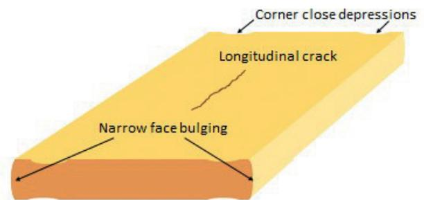
Fig. 2 - Corner close depressions combined with narrow face bulging and long cracks
