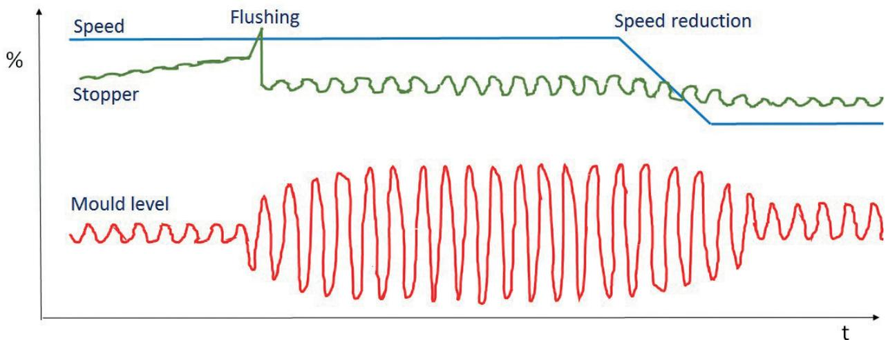
**Fig. 7** - Stopper position, mould level and casting speed in case of fluctuation.
