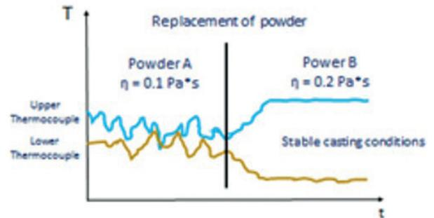
**Fig. 6** - Thermo-diagrams in case of mould powder replacement by a more viscous one.
