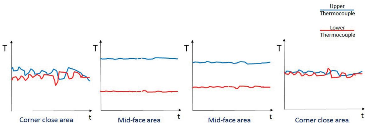
Fig. 4 - Temperatures thermocouples close to the corner and in the centre area
