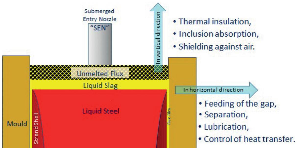
Fig. 1 - Functions of mould flux in vertical and horizontal direction.
