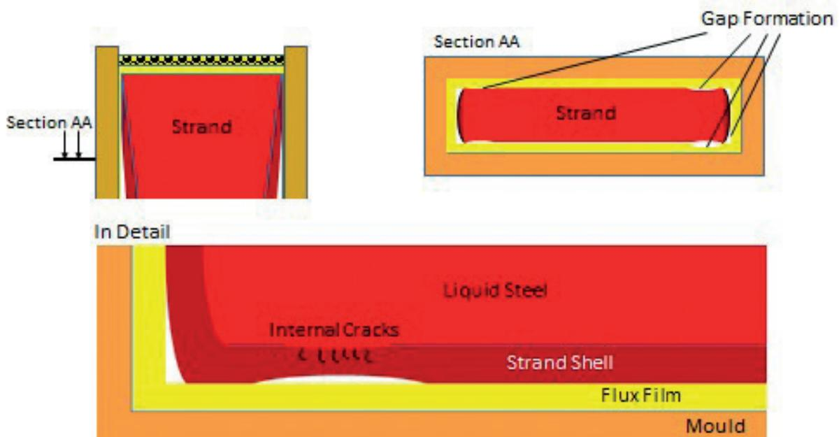
Fig. 3 - Mechanisms of narrow face bulging and formation of corner close depressions
