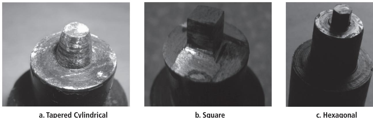
**Fig. 1** - Tool Pin Profile of the FSW tool
