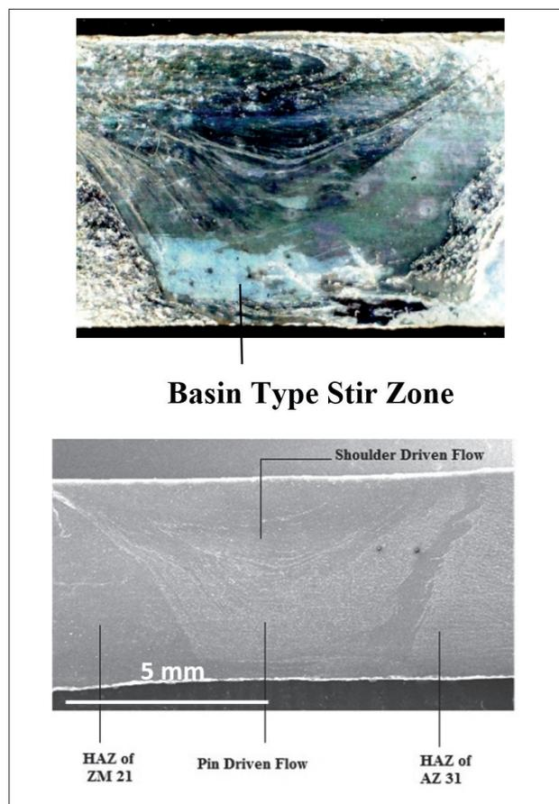
**Fig. 4** - Macro Structure of the weld
