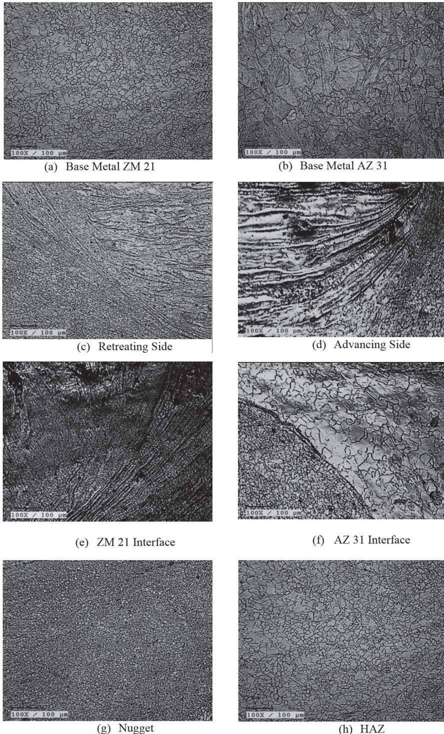
**Fig. 5** - Micro Structure of the weld at different location
