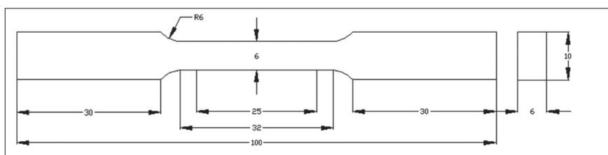
**Fig. 2** - Dimensions of tensile specimen
