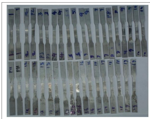
**Fig. 3** - Photograph of EDM Wire Cut Tensile Samples
