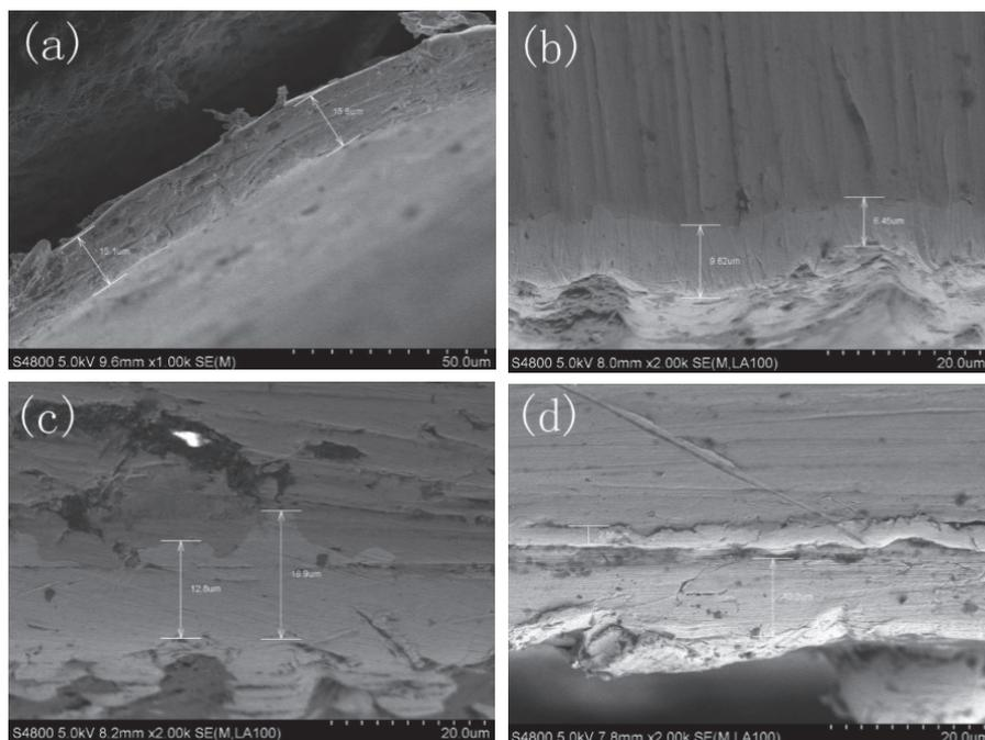
**Fig. 6** - Cross section SEM microstructure of different pretreatments
