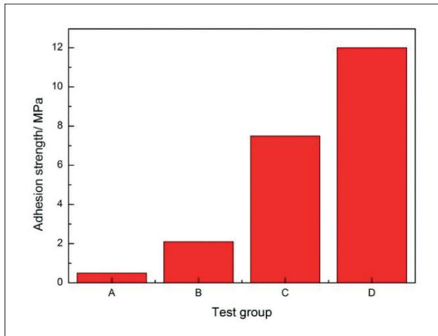
**Fig. 3** - Coating adhesion strength of different pretreatment process
