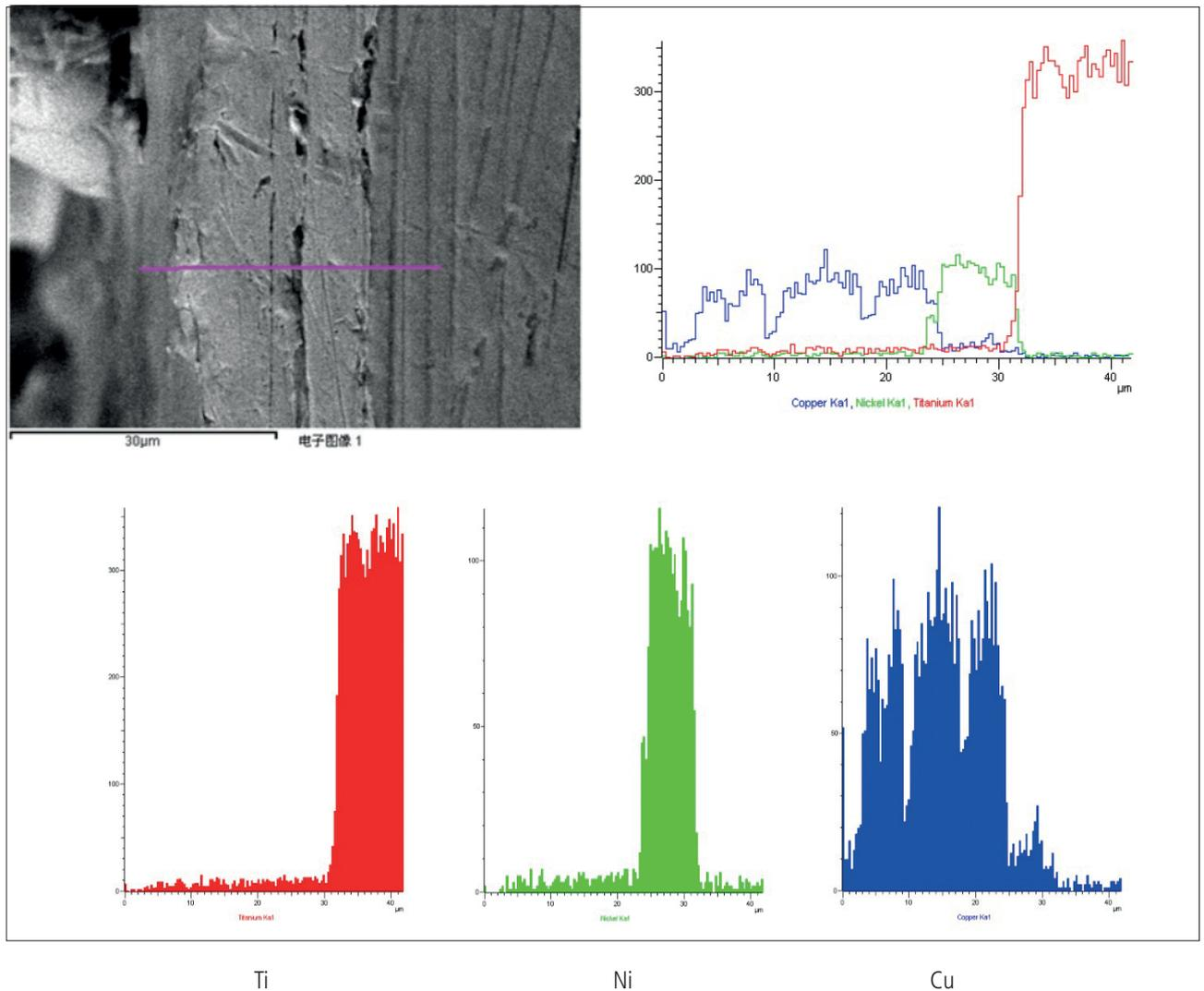
**Fig. 7** - EDS results of Cu coating in group D
