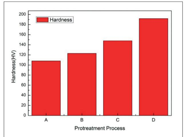
**Fig. 4** - Copper plating micro-hardness of different pretreatments
