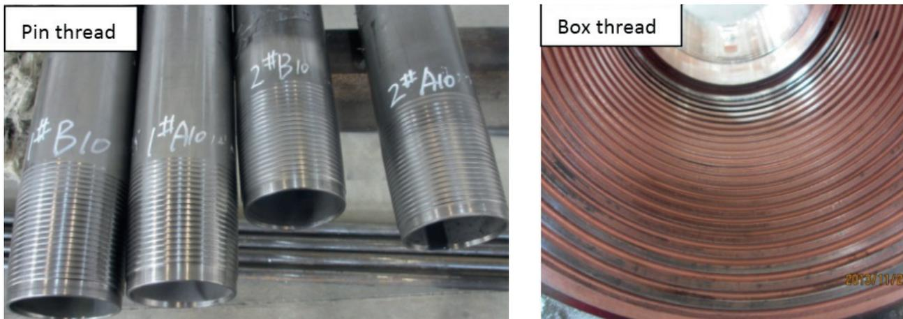
**Fig. 9** - Morphology of titanium thread after 10-times make-up and break-out tests with group D treatment
