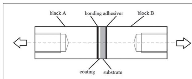
**Fig. 1** - Schematic diagram of coating bond strength test sample
