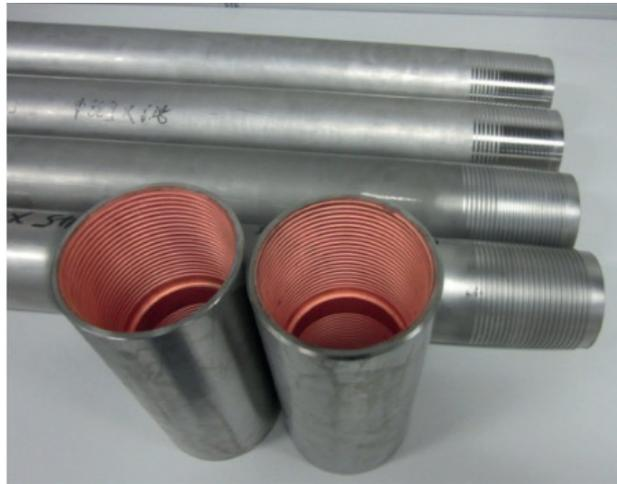
**Fig. 8** - TC4 titanium alloy tubing connection samples with Cu coating in make-up/break-out tests
