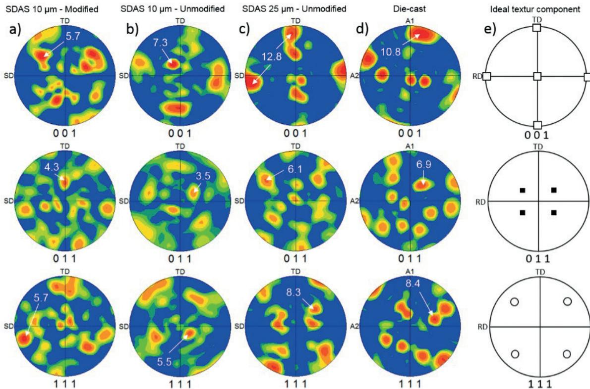
**Fig. 2** - a-d) Experimental pole figures of each case. e) Standard pole figures showing ideal texture components. SD is solidification direction, TD is transversal direction.
