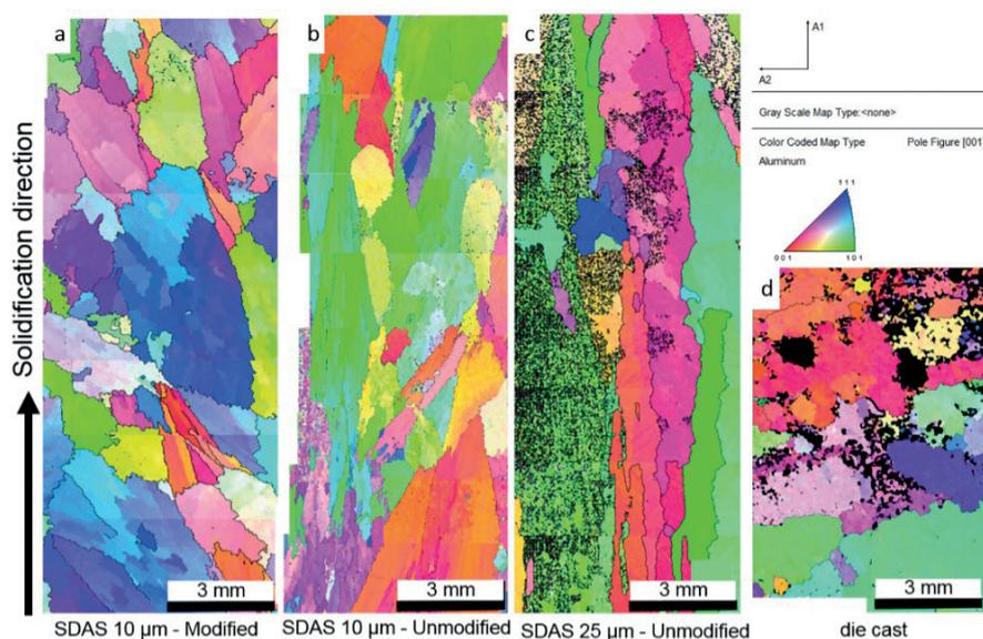
**Fig. 1** - Composite EBSD map taken from the center of cast specimens.
