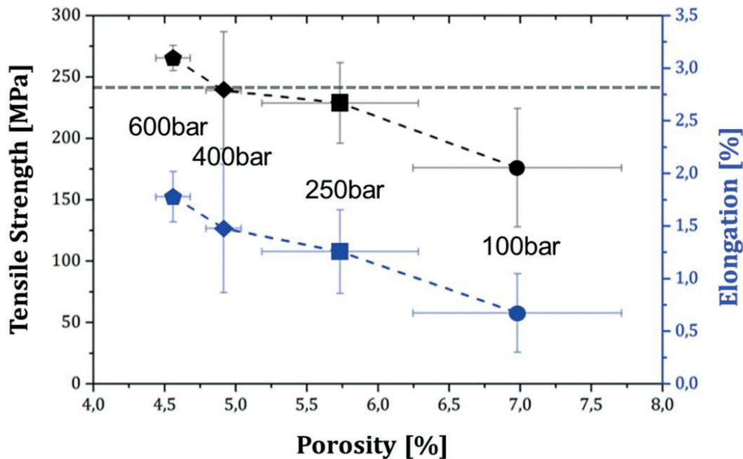
Fig.2 - Mechanical Properties related to cast part porosity
