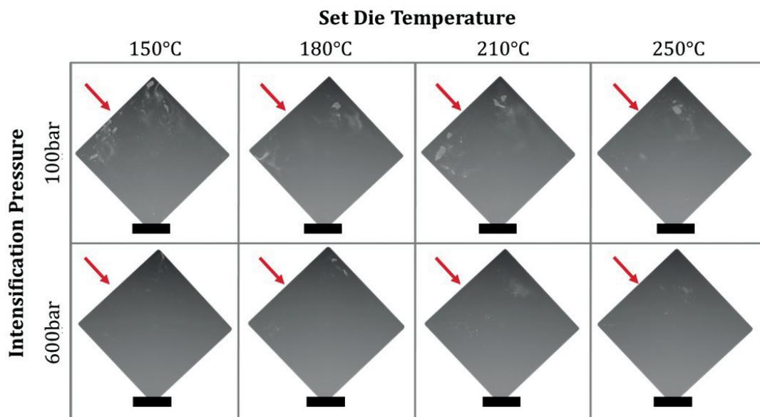
**Fig.1** - Porosity distribution within the cast part
