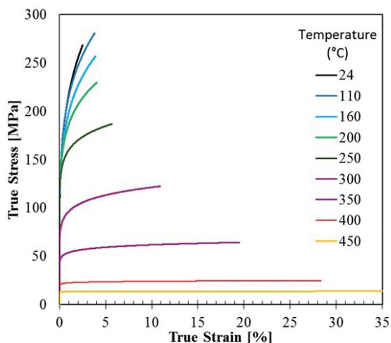
**Fig. 1** - Overview of the true stress-strain curves in tension tests at different temperatures in the range 24-450°C for EN-AC 46100 alloy.
