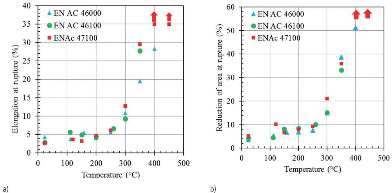
**Fig. 3** - Elongation at rupture (a) and reduction of area at rupture (b) plotted as functions of test temperatures for the three investigated alloys.
