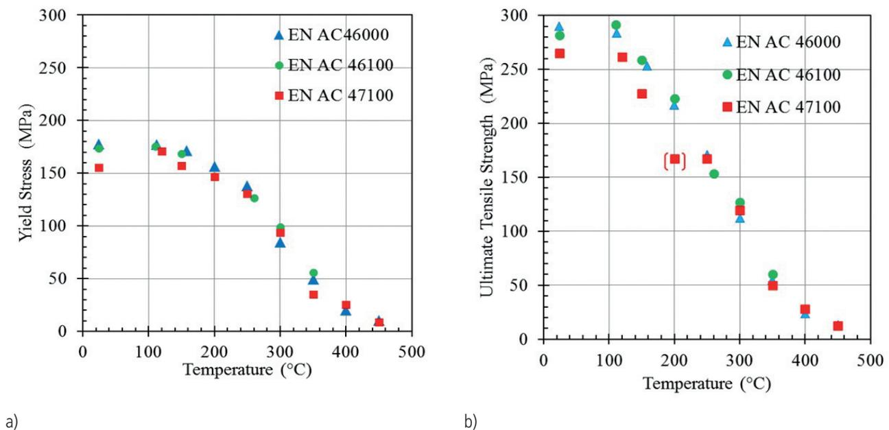
**Fig. 2** - 0.2% offset Yield Stress (a) and Ultimate Tensile stress (UTS) (b) plotted as functions of test temperatures for the three investigated alloys. The point in square brackets corresponded to an anomalous rupture.
