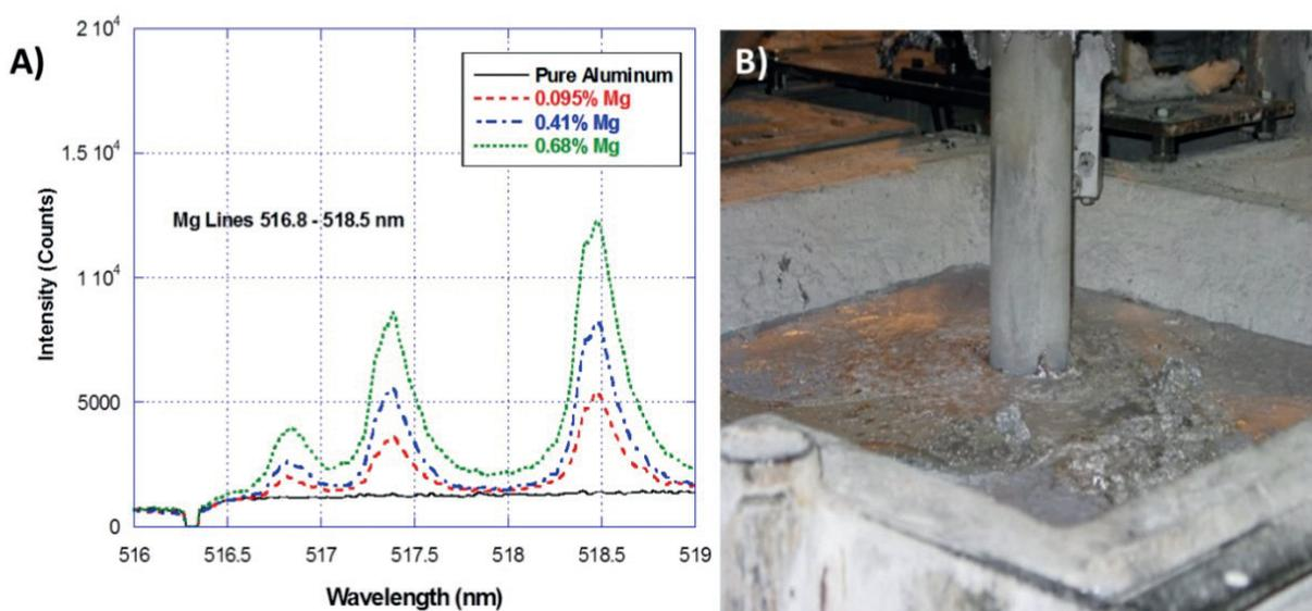
Fig. 2 - (A) Change in LIBS spectrum with addition of magnesium to molten aluminum [5]; (B) Detail of immersed probe over filter bowl [3].
