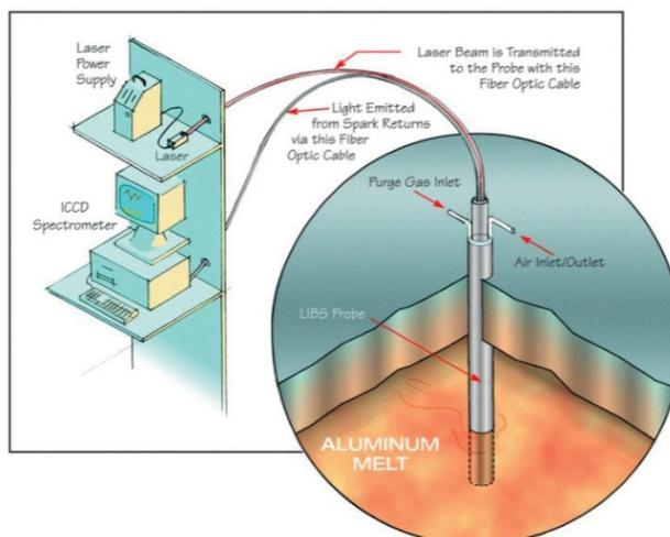
Fig. 1 - Schematic of an immersed LIBS probe [4].
