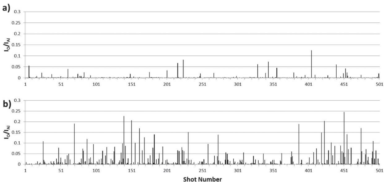
**Fig. 4** - Normalized Oxygen Peak Intensity vs. Laser Shot Number for (A) Base Al; (B) Dirty Al [6].
