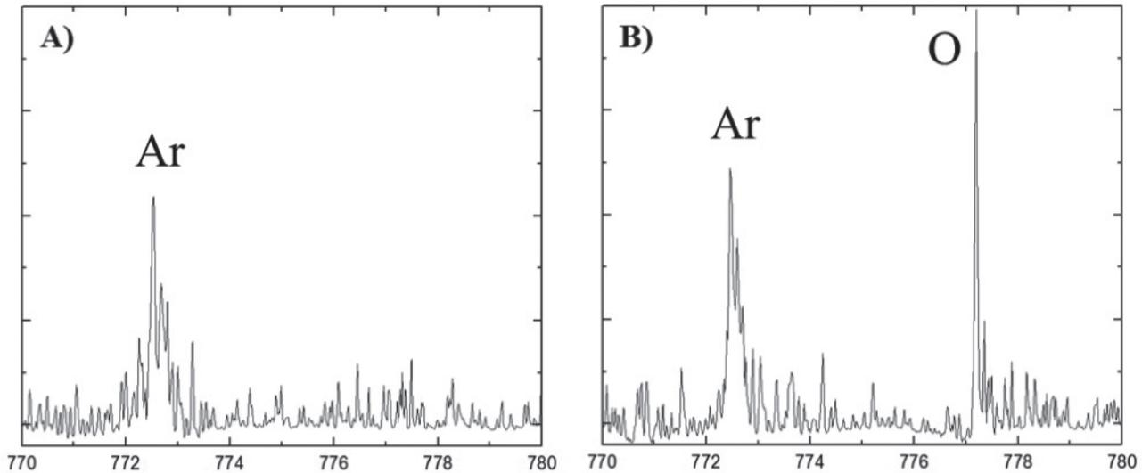
**Fig. 3** - Example of LIBS spectra of molten aluminum with (A) no oxide hit and (B) with an oxide hit. The argon peak near 772 nm is from the bubbling gas [7].
