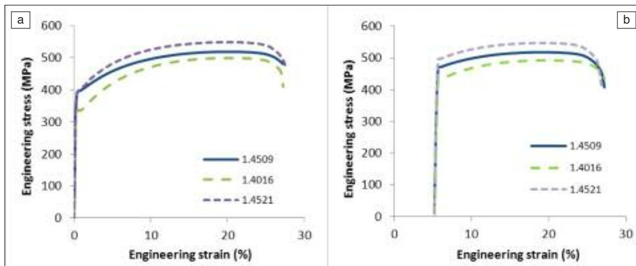
FIG. 2 Typical stress-strain curves in the as-received condition a) and after prestraining (b).
