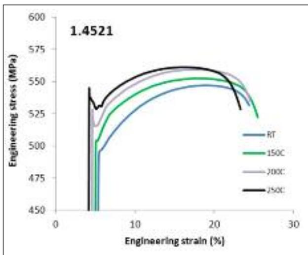
FIG. 4 **Stress-strain curves for 1.4521 aged at different temperatures. Curves have been displaced by 0.40% along the abscissa to avoid crowding.**
