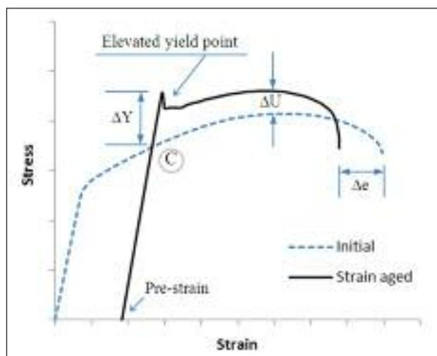
**FIG. 1** *The influence of strain aging on the stress-strain curve of skin-pass rolled steel. The elevated yield point is restored, both yield and tensile strength increase by  $\Delta Y$  and  $\Delta U$ , respectively, and the total elongation decreases by  $\Delta \epsilon$ . In the absence of strain aging, the stress-strain curve of the pre-strained material would join the initial curve at the point C.*
