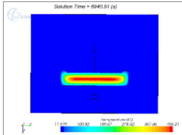
**Fig. 17** *Steam generator tubesheet thermal field at 7000 s in forced convection.*
