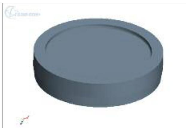
**FIG. 2** *Steam generator tubesheet.*
