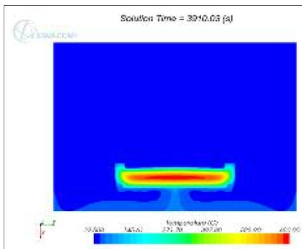
**FIG. 11** **Steam generator tubesheet: thermal field at end simulation.**
