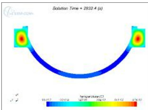
**Fig. 9** **Reactor vessel closure head: thermal field at end simulation.**
