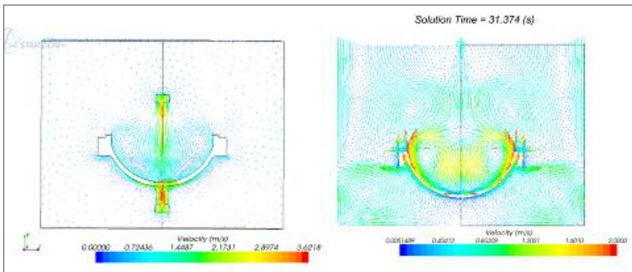
**FIG. 13 Comparison between water vector fields in natural convection (right) and forced convection (left).**
