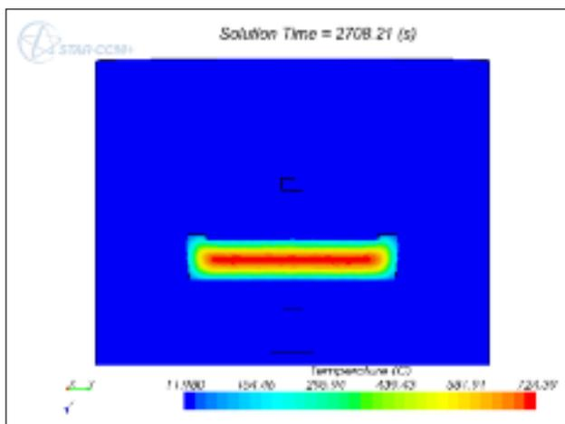
**FIG. 16** *Steam generator tubesheet thermal field at 3000 s in forced convection.*
