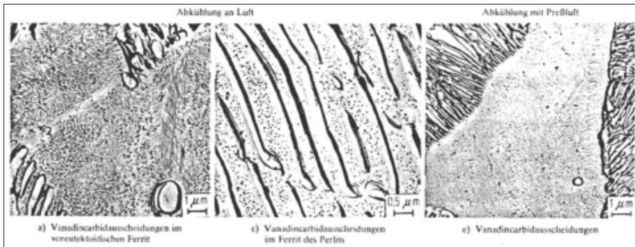
**FIG. 8** *TEM of extraction replica showing VCN precipitates in both proeutectoid and pearlitic ferrite. Steel Ck45 + 0.1%V, air cooled from forging temperature 1250 °C, 50mm. [3]*
