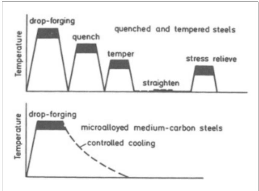
loped to replace heat treated carbon and low alloy steels. As shown in Figure 11, [7] the processing of these microalloyed forgings is quite streamlined, when compared to the normal heat treatment route. At least four processing steps can be avoided, plus the cost of handling and transporting the forgings. Furthermore, the problem of mixed steel is much less likely in such a streamlined process. The economic benefits of this simple process are clearly evident.
