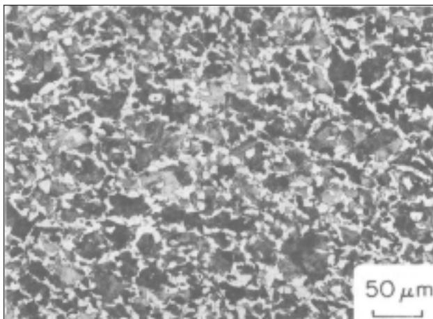
FIG. 2 **Ferrite-pearlite optical microstructure exhibited by the as-received 1045V steel. Transverse section.[6]**
