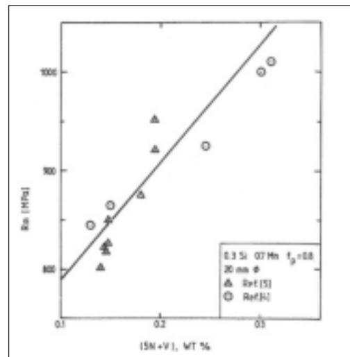
**Fig. 7** *The effect of precipitation hardening by V and N on Yield strength [4,1]. All data have been normalized, using Eq. (1), to 0.3Si, fp=0.8 and a section size of 20 mm Φ. All Steels contain 0.7Mn and were austenized at 1200-1250 °C [6]*
