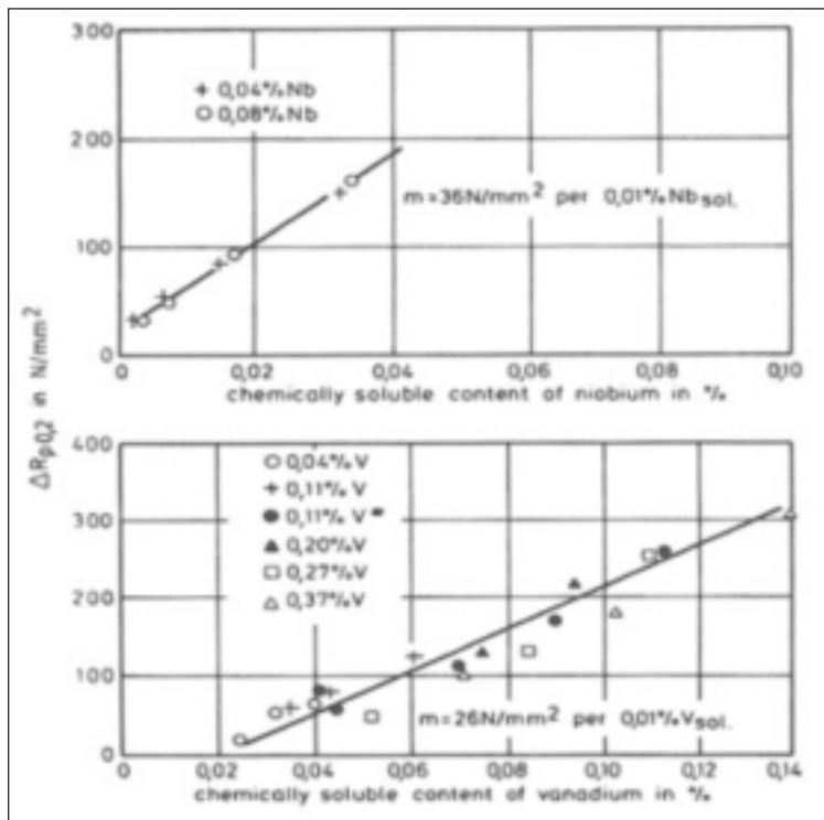
**FIG. 6** *Precipitation hardening effect of V and Nb. Austenizing: 800-1300°C, 0.5hr air cool (\* 0.11%V ~ Compressed air cool). [7]*
