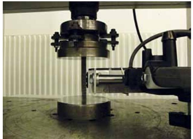
**Fig. 2 - Measuring jig for applying compression. Since the test piece had a tendency to buckle the test piece was shortened to 100 mm length**
