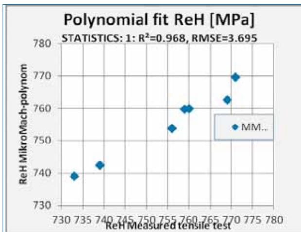
**Fig. 9 - Polynomial fit, yield strength, ReH 3mm EHS-steel**
