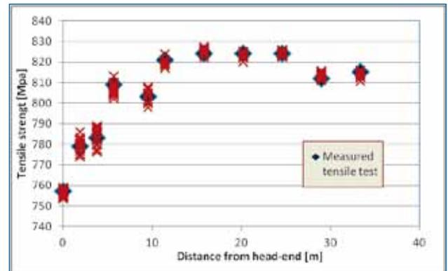
**Fig. 8- Measured test samples head end EHS-steel strip**
