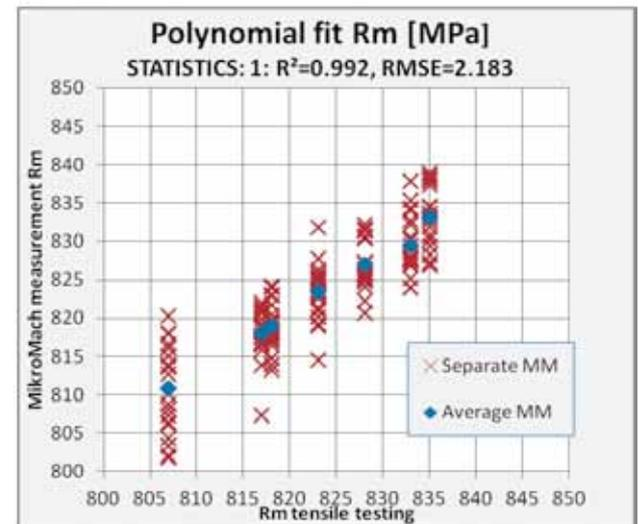
**Fig. 10 - Polynomial fit tensile strength, Rm 3 mm EHS-steel**
