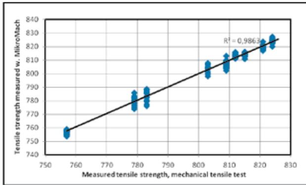
**Fig. 7 - Repetition accuracy, tensile strength**
