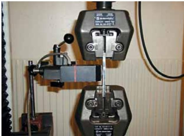
**Fig. 1 - Measuring jig for applying tensile stress during calibration**
