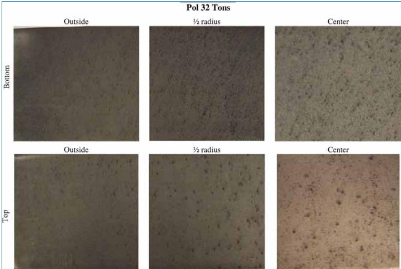
**Fig. 9 - Macrostructure standard ingot (HCl 50% etch)**
