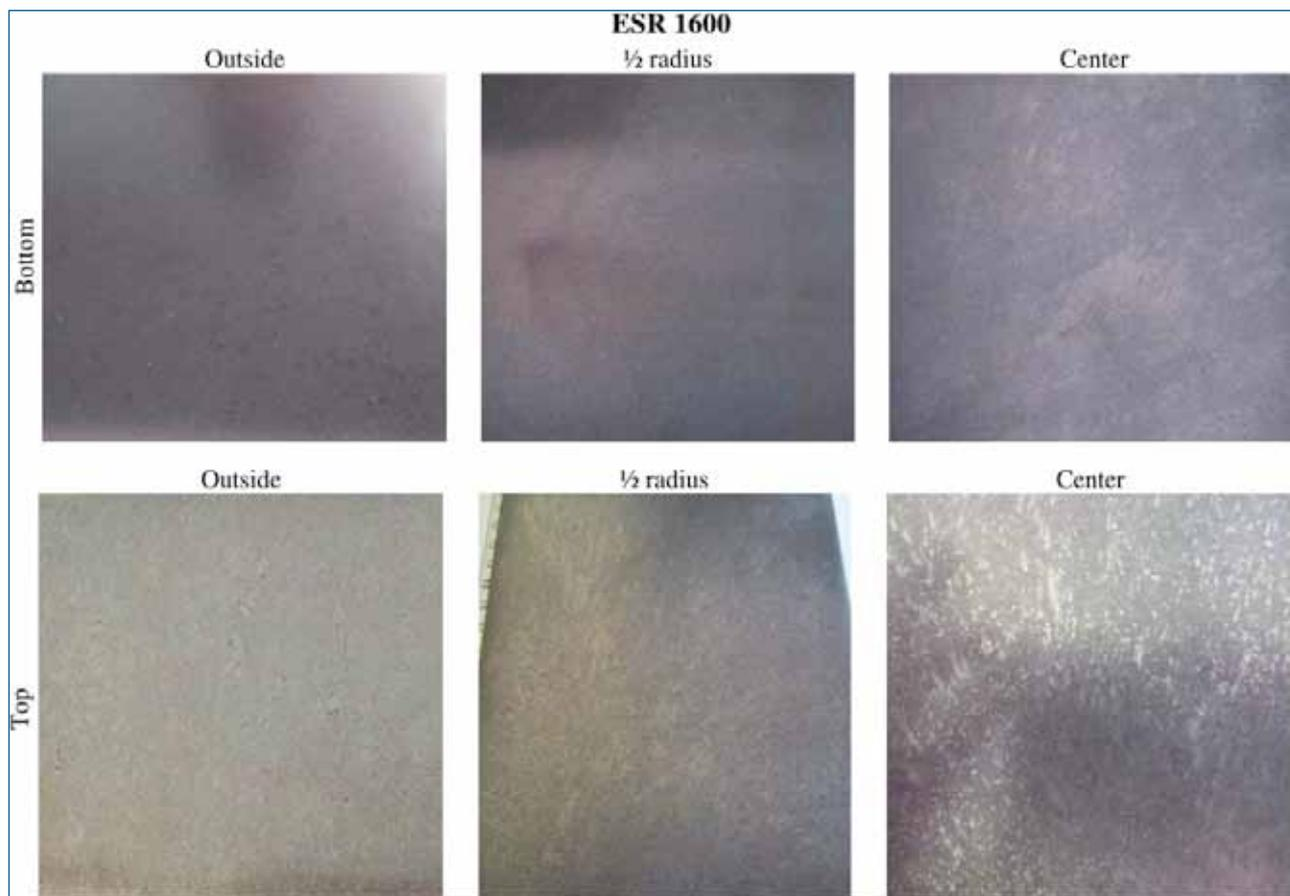
**Fig. 8 - Macrostructure ESR ingot (HCl 50% etch)**
