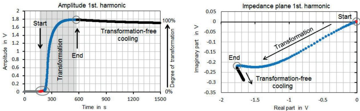
**Fig. 4** - Evolution of the 1<sup>st</sup> harmonic for sample 1, which featured a bainitic microstructure with scaling after the transformation
