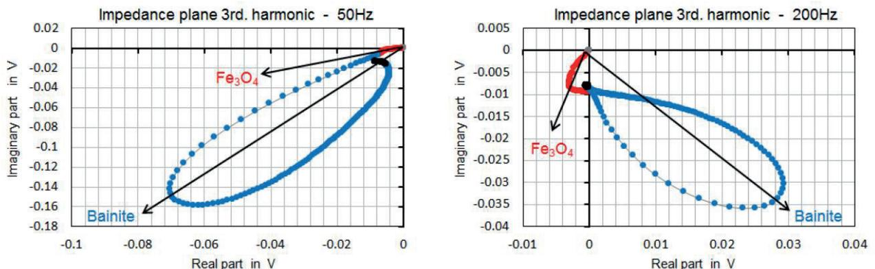
**Fig. 5** - 3<sup>rd</sup> harmonic for sample 1 upon a transformation to a bainitic microstructure along with formation of scaling for two different test frequencies
