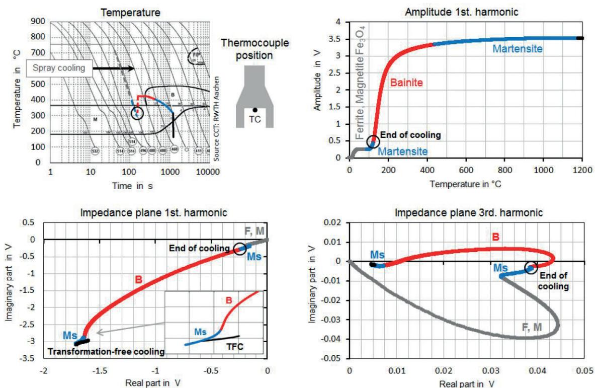
Fig. 10 - Temperature-time-path and signal evolution for sample 6 - "Stepped Shaft"
