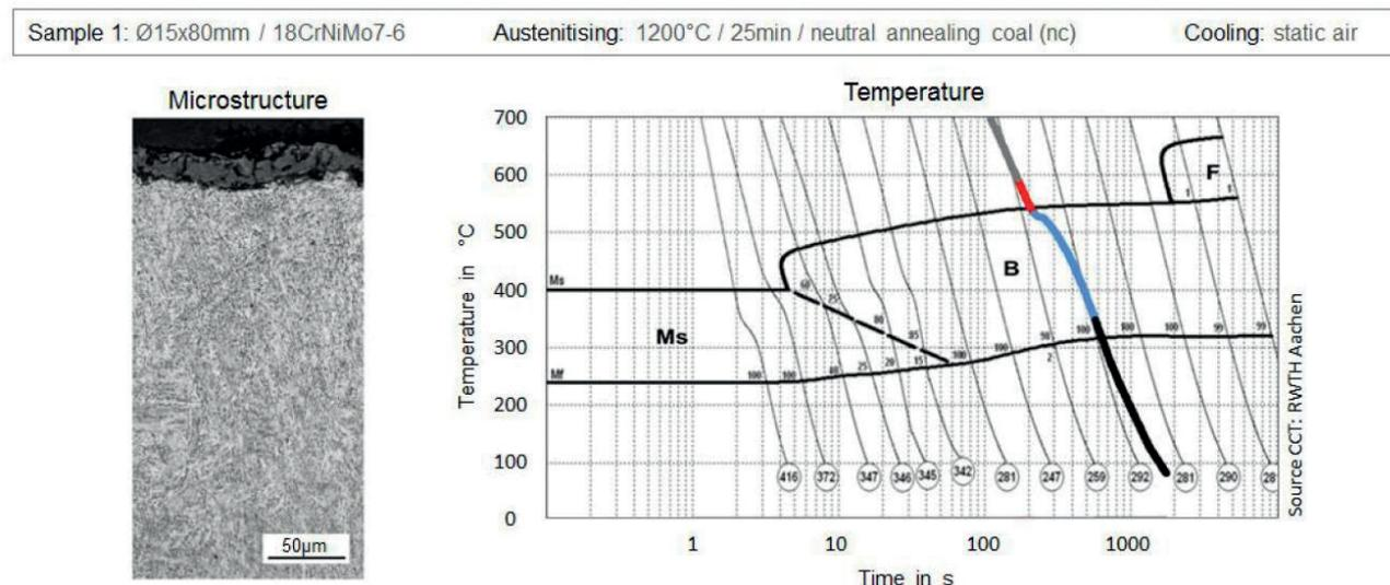
Fig. 3 - Optical micrograph of the bainitic microstructure along with scaling at the outer surface (left) and temperature-time-profile of sample 1 (right)
