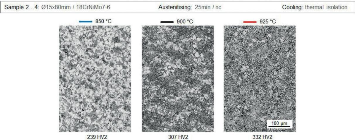
Fig. 7 - Optical micrographs of the microstructures formed in samples 2, 3 and 4
