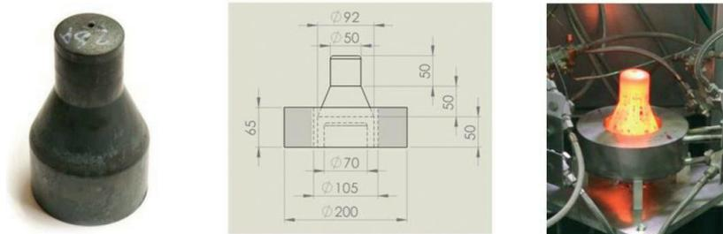
Fig. 9 - Demonstration component "stepped shaft" and experimental setup in the spray-field
