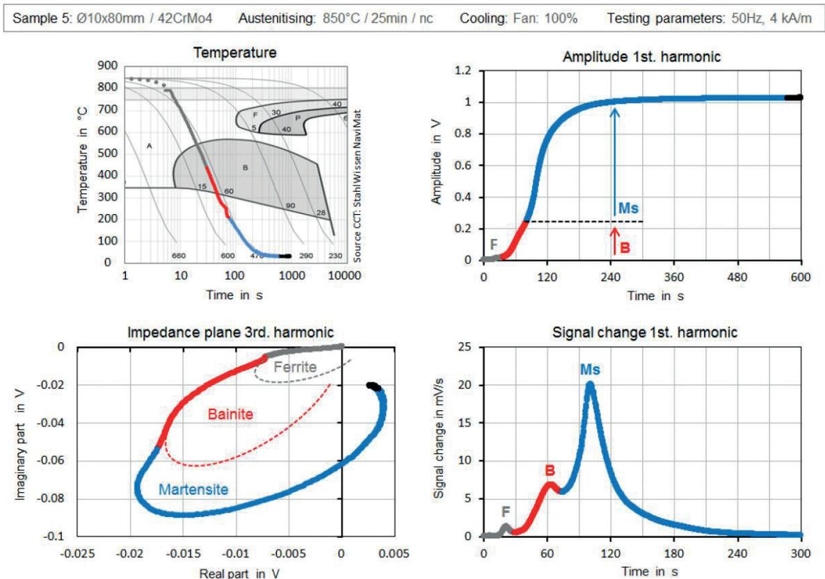
Fig. 8 - Temperature-time-path and evolution of the measured signal for sample 5 with a bainitic-martensitic microstructure
