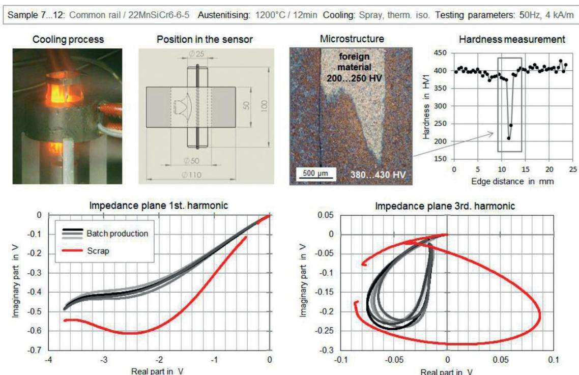
**Fig. 11** - Demonstration component “common rail” and signals recorded for samples 7 to 12, see main text for details , partly recomplied from [7]
