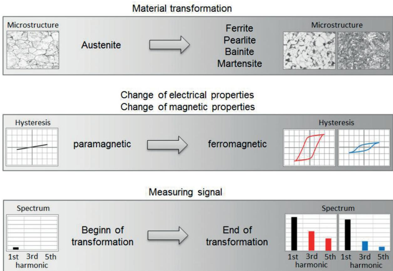
Fig. 1 - Measuring principle, see main text for details
