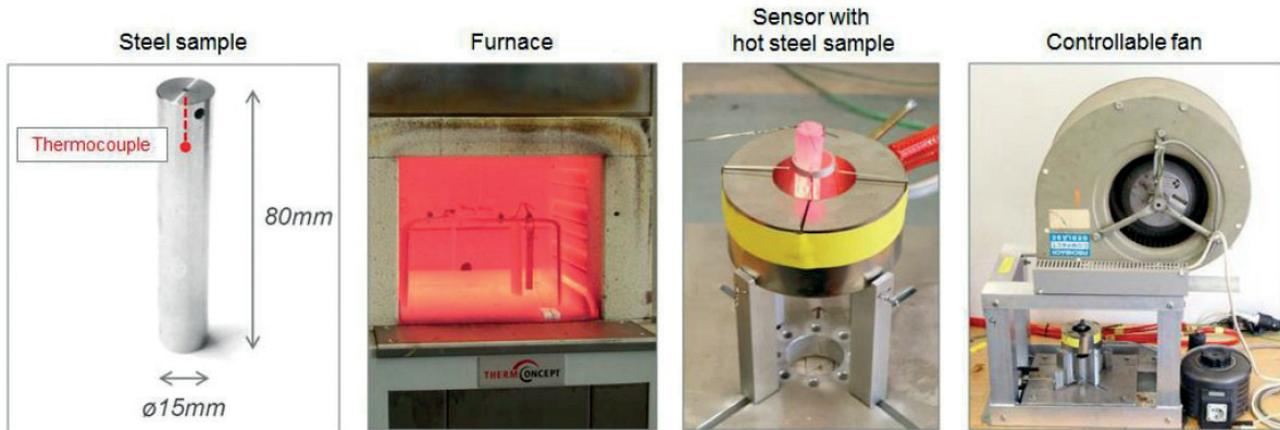
Fig. 2 - Experimental setup for cylindrical steel samples
