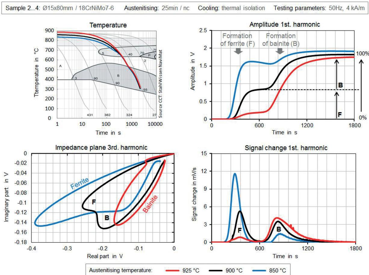
**Fig. 6** - Temperature and signal courses of the samples 2, 3 and 4 with different ferritic-bainitic microstructures, partly recomplied from [7]
