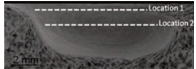
FIG. 1 A macrograph of the FSPed region showing two locations where the microhardness data were collected.
