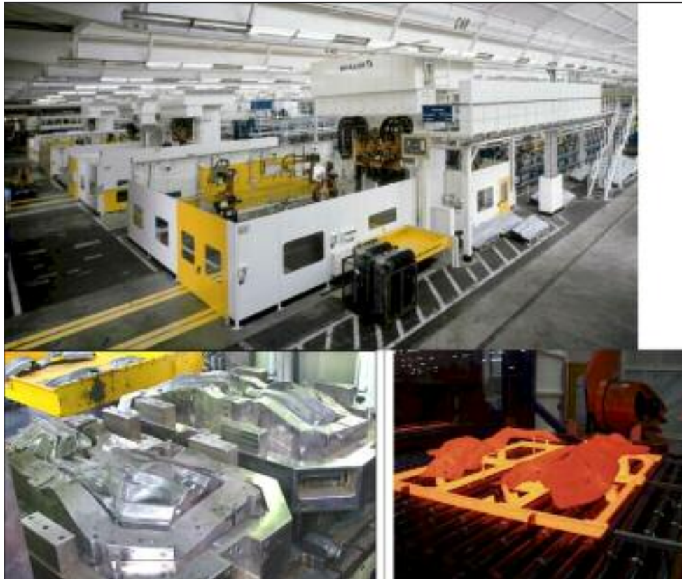
FIG. 1 Hot Stamping line, dies, and pieces coming out of the furnace (indirect process) at VOLKSWAGEN AG Kassel's plant.
