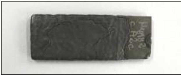
FIG. 3 Steel strip after dipping experiment.
