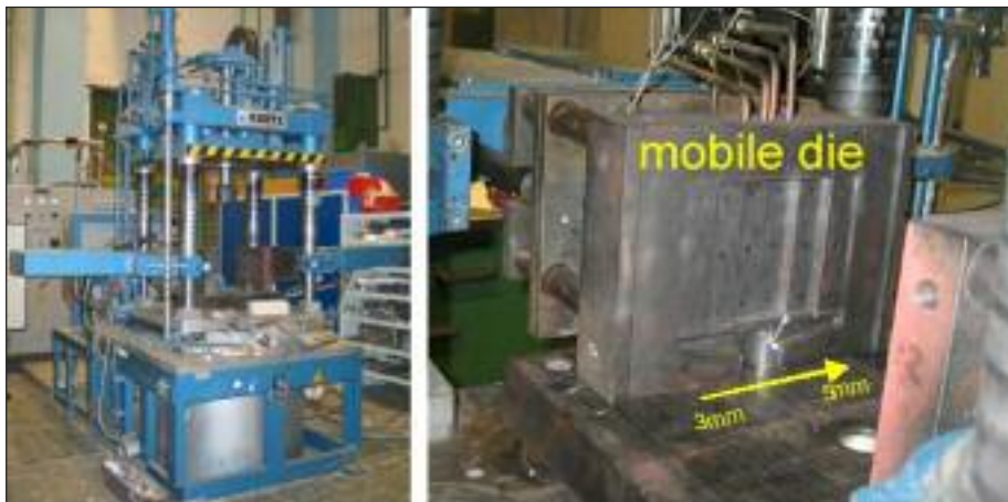
FIG. 2 LPDC machine and the experimental die (cooling channels).
