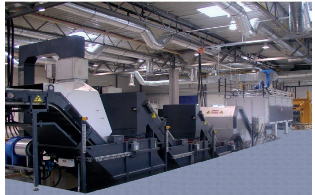
Fig. 8 - Conveyor belt furnace with salt bath and washers
