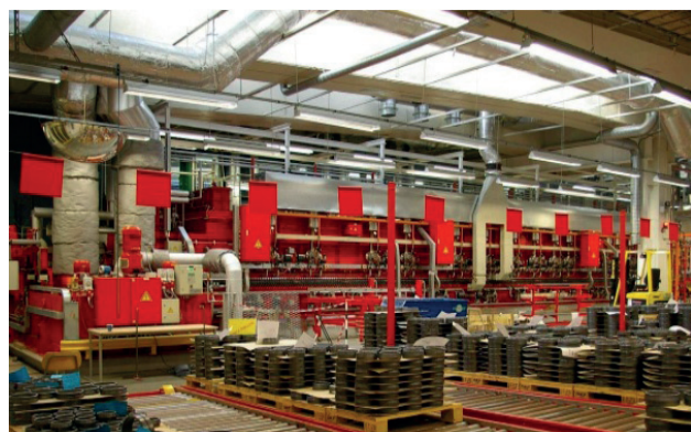
Fig. 5 - Austenitizing furnace of a roller hearth furnace line
