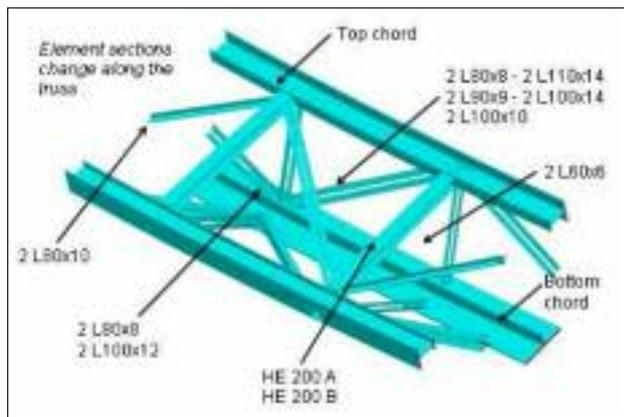
**FIG. 3** Section of the bridge deck of "Ponte del Mare".
