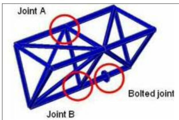
**FIG. 4** Re-designed bridge deck with tubular sections made of HSS.
