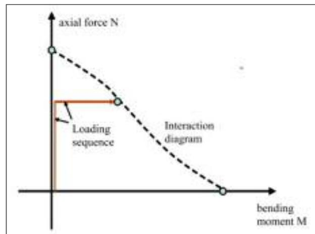
**FIG. 6** Interaction diagram and loading sequence for member tests under monotonic loading.
