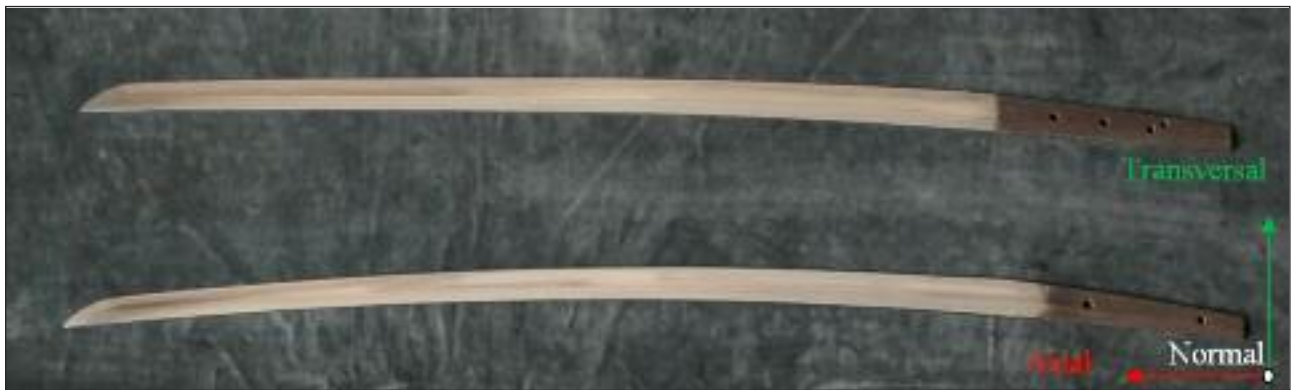
FIG. 1 Pictures of the Bizen Sue-Aoe tachi blade (upper) and of the Mino Kanesada katana blade. It is evident the presence of some holes in the tang testifying the modification of the original length. The curvature of the two swords is also very different. The directions of the strains measured on ENGIN-X are also shown.
