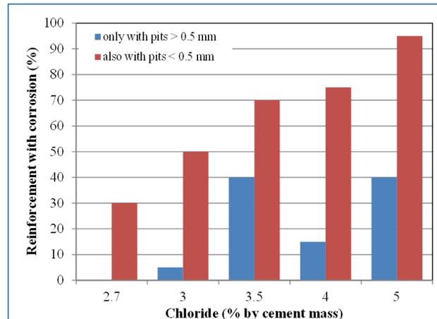
**Fig. 3 – Number of bars (%) with pitting corrosion initiation after 24 hours anodic polarisation test at +200 mV vs SCE.**
