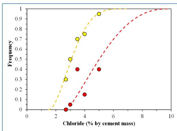
**Fig. 4 – Cumulative probability distribution function (fitted by a Beta distribution) of the 1.4362 steel determined from experimental results of the anodic polarisation tests at +200 mV vs SCE (indicated with the points in figure) considering only macro-pits (in red) and also micro-pits (in yellow).**
