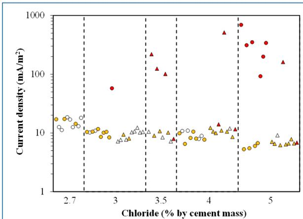
**Fig. 2 – Current density measured at the end of the 24 hours of polarisation at +200 mV vs SCE on the bars in concrete (circle symbols) and mortar (triangle symbols) specimens with different chloride contents (white symbols = no corrosion observed on steel surface; red symbols = pits of dimension higher than 0.5 mm observed on steel surface; yellow symbols = small pits of dimension lower than 0.5 mm observed on steel surface).**
