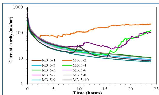
**Fig. 1 – Current density of the bars of 1.4362 stainless steel in mortar specimens with 3.5% Cl<sup>-</sup> by cement mass, during the 24 hours of polarisation at +200 mV vs SCE.**
