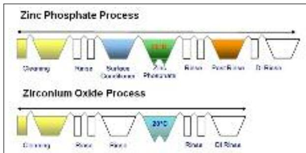
**FIG. 3** Comparison of a traditional Zinc Phosphating process sequence to the much shorter zirconium oxide type o conversion coating.
