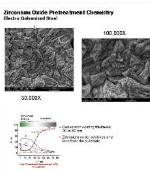
FIG. 2 Typical coating composition and film thickness (XPS, bottom), and FE-SEM micrographs (top) of a zirconium oxide coating.
