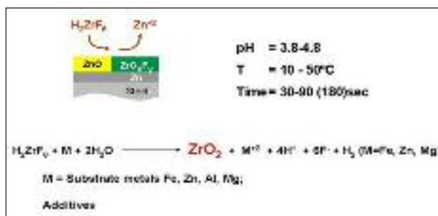
FIG. 1 Simplified conversion coating formation mechanism.
