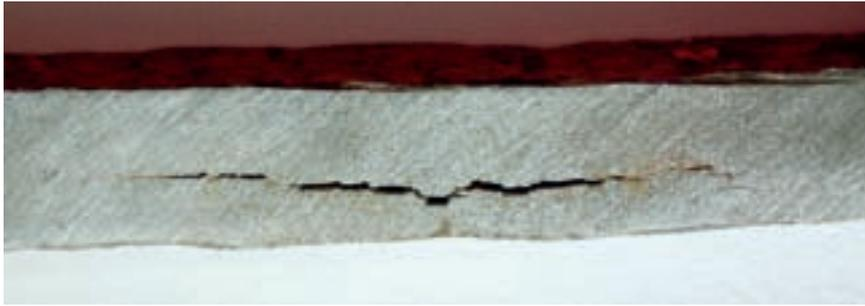
**Fig. 1 – Stepwise cracking due to hydrogen diffusion inside an ASTM A 516 Gr. 70 steel plate.**
