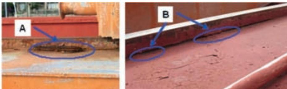
**Fig. 4 – Corrosion damage in a bridge crane: crevice (A) and corrosion fatigue (B)**
