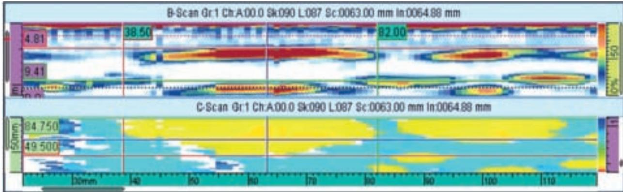
**Fig. 2 – Ultrasound measurements performed by the Phased-Array method with linear scanning. B scan is the sectional view and C scan is the plan view. According to the colored scale, the measured crack was 43.5 mm long, 35.2 mm wide and has a depth of 4.8 mm with a wall thickness of 9.4 mm.**
