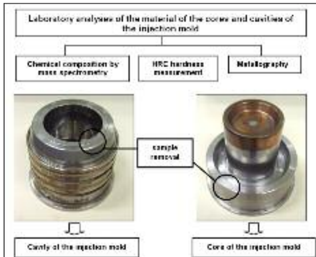
FIG. 1 Laboratory analyses of cores and cavities of the injection mold.
