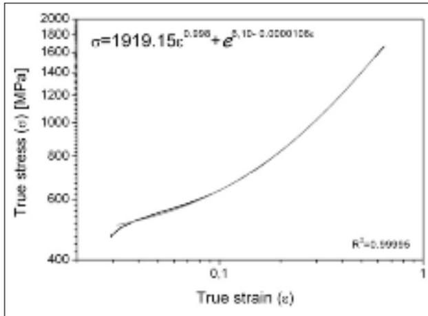
**FIG. 3** True stress-true strain diagram of the Fe-25Mn-0.3C-0.4N. The black line represents the measured data and the grey line the fitted line according to Ludwigson relation. The equation corresponds to the regression from the Ludwigson relation.
