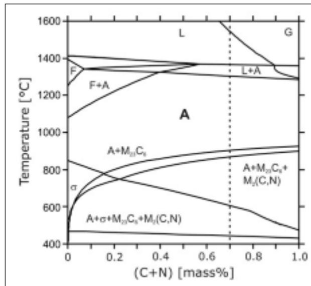
FIG. 1 Phase diagram of the system Fe-20Mn-12Cr-C-N (C/N=0.75).
