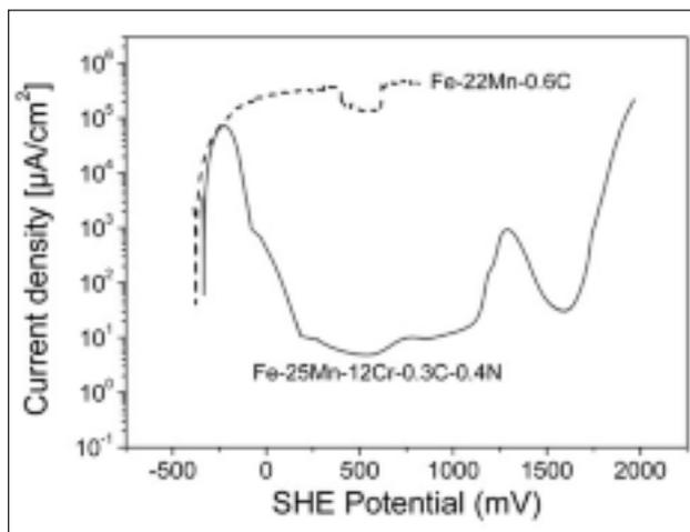
**FIG. 6** Current potential diagram of the steels Fe-25Mn-12Cr-0.3C-0.4N and Fe-22Mn-0.6C in 0.5M H<sub>2</sub>SO<sub>4</sub> solution [2].
