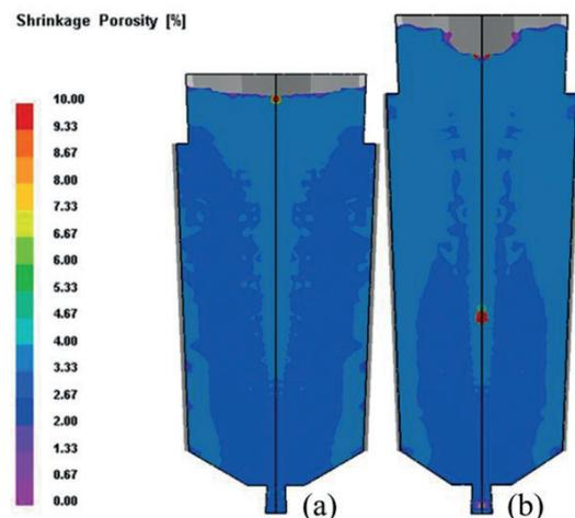
**Fig. 5** - Effect of the H/D ratios on the shrinkage porosity of the ingot: (a) 1#, (b) 2#
