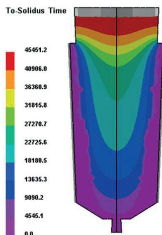
Fig. 1 - Contour line of solidification time in 19 ton ingot
