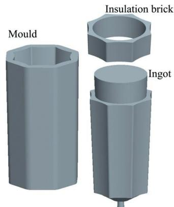
**Fig. 2** - The geometry of the 19 ton steel ingot and the mould
