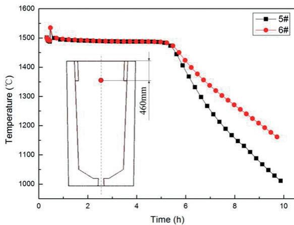
**Fig. 9** - Simulated cooling curves of the position in the bottom of the hot top of two ingots with insulation height of 410mm and 510mm respectively (5# and 6#)
