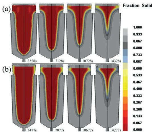
**Fig. 4** - Distribution of solid fraction during the solidification of the ingot with different H/D ratios: (a) 1#, 2.00, (b) 2#, 2.45
