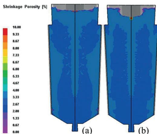
**Fig. 7** - Effect of taper on the shrinkage porosity of the ingot: (a) 3#, (b) 4#
