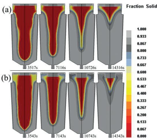
**Fig. 6** - Distribution of solid fraction during solidification of the ingot with different tapers: (a) 3#, 6.76%, (b) 4#, 9.15%
