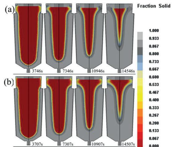
**Fig. 8** - Distribution of solid fraction during solidification of the ingot with different height of insulations: (a) 5#, 410 mm, (b) 6#, 510 mm
