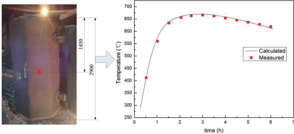
**Fig. 3** - Comparison of the calculated temperature with the measured one on the mid-point of the mould wall of the 19t 1.2738 ingot
