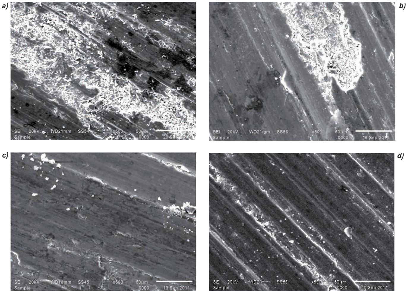
**Fig. 7 - SEM photo micrographs of Al-7Si-0.45Mg alloy wear pins (a) without grain refiner and with 1.4 wt. % of grain refiners (b) Al-5Ti-1.25C (c) Al-5Ti-0.8C and (d) Al-5Ti-1B**
