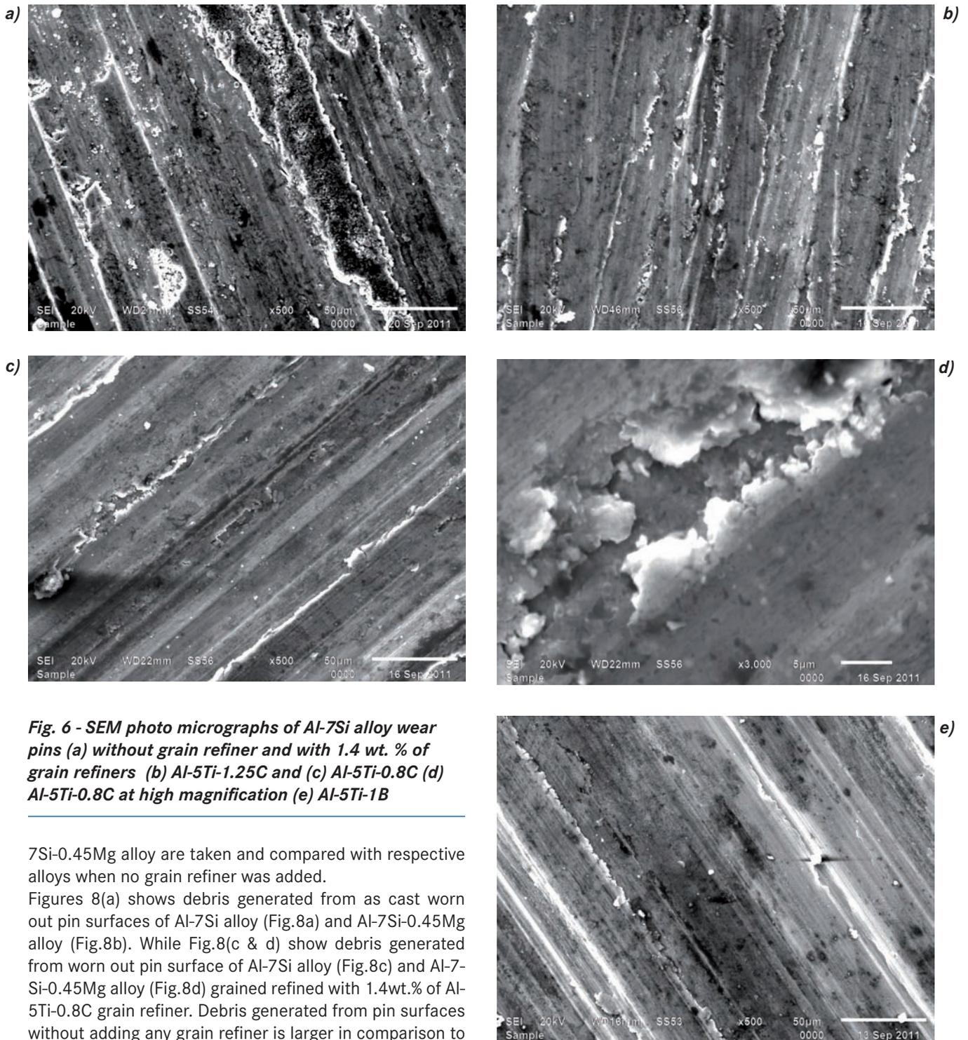
**Fig. 6 - SEM photo micrographs of Al-7Si alloy wear pins (a) without grain refiner and with 1.4 wt. % of grain refiners (b) Al-5Ti-1.25C and (c) Al-5Ti-0.8C (d) Al-5Ti-0.8C at high magnification (e) Al-5Ti-1B**
