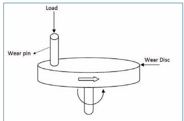
Fig. 1 - Schematic representation of the pin-on-disc wear monitor
