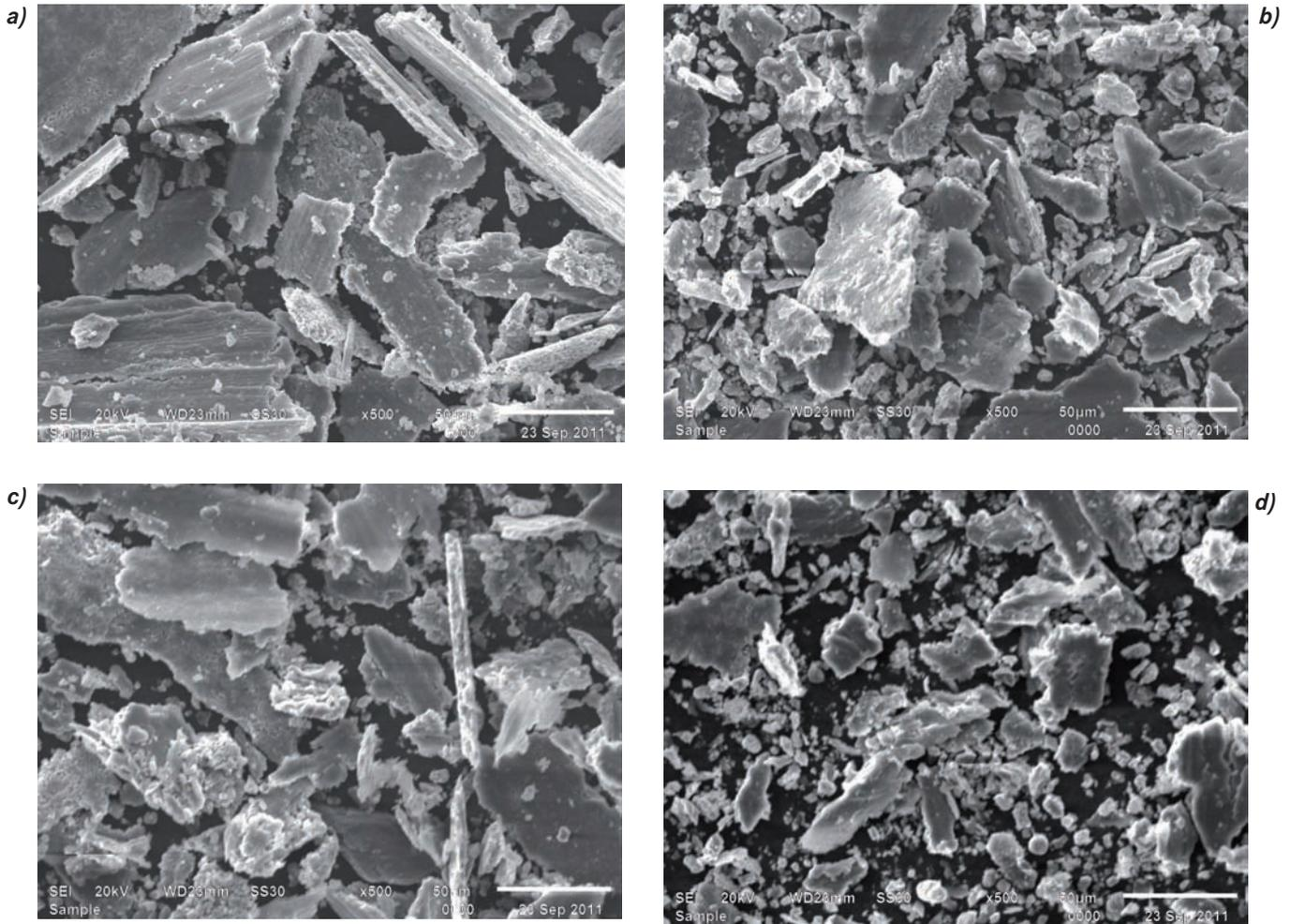
**Fig. 8 - SEM photo micrographs of debris (a) Al-7Si alloy without grain refiner (b) Al-7Si alloy grain refined with 1.4 wt. % of Al-5Ti-0.8C master alloy (c) Al-7Si-0.45Mg alloy without grain refiner (d) Al-7Si-0.45Mg alloy grain refined with 1.4 wt. % of Al-5Ti-0.8C master alloy**
