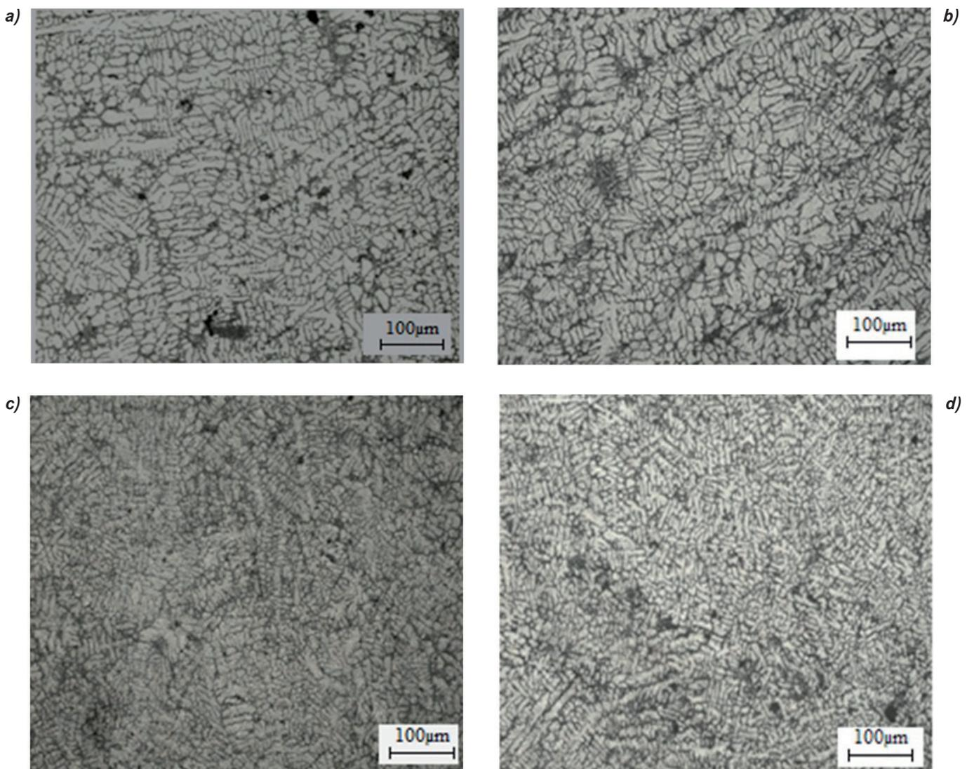
**Fig. 2 - Microstructure of Al-7Si alloy without addition of grain refiner (a) at 0 min. and with addition of 0.2wt. % of (b) Al-5Ti-1.25C (c) Al-5Ti-0.8C (d) Al-5Ti-1B grain refiners at 2 mins. of holding time.**
