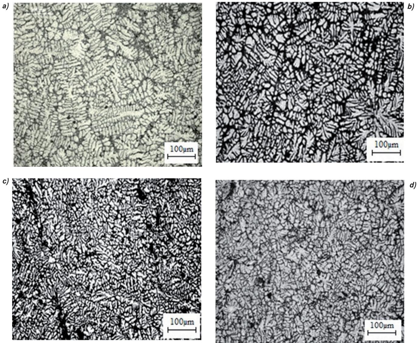
**Fig. 3 - Microstructure of Al-7Si-0.45Mg alloys without addition of grain refiner at (a) 0 min. and with addition of 0.2wt% grain refiner of (b) Al-5Ti-1.25C (c) Al-5Ti-0.8C (d) Al-5Ti-1B at 2 mins. of holding time.**
