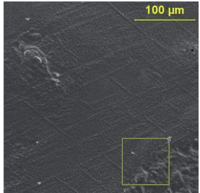
**Fig. 11 - SEM image showing dendritic fracture surface with thin film**
