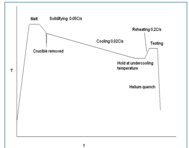
Fig. 6 - Thermal path for undercooling experiments
