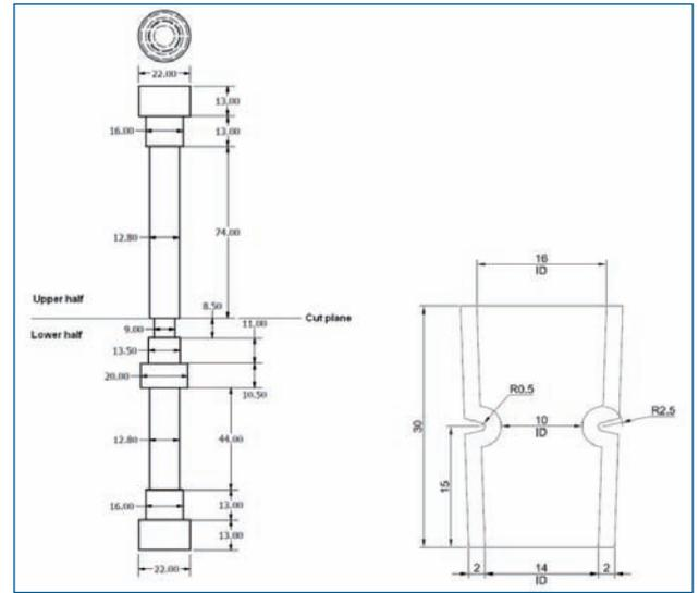
**Fig. 1 - Sample and crucible dimensions for this work**
