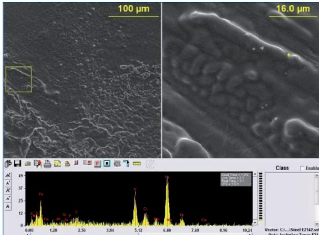
**Fig. 12 - Showing EDS analysis of V(C,N) precipitate**
