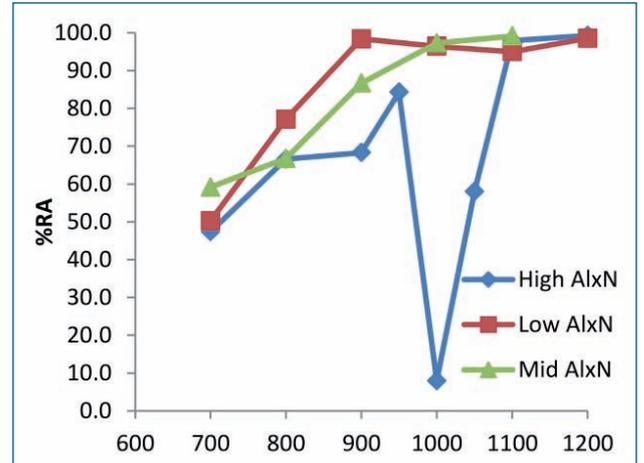
Fig. 4 - Results of direct cooling to test temperature experiments for P20 with varied aluminum and nitrogen
