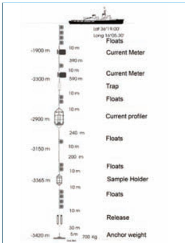
Figure 1: Mooring line used in field tests.
