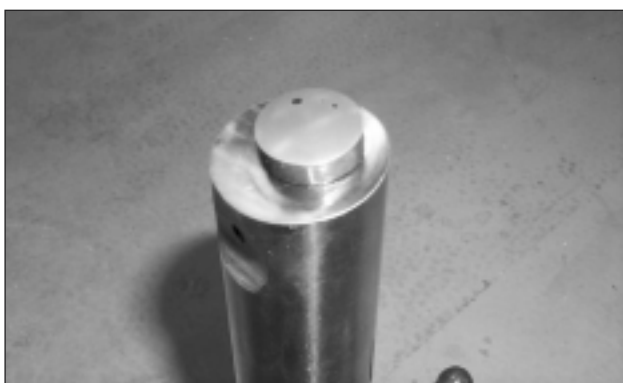
FIG. 6 The test pin with one large and one small wear mark.
