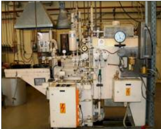
FIG. 2 The Ipsen RT25-EM sealed quench furnace used for the heat treatment.
