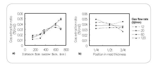
argon gas extracted from mold meniscus is measured by water model and commercial caster.
