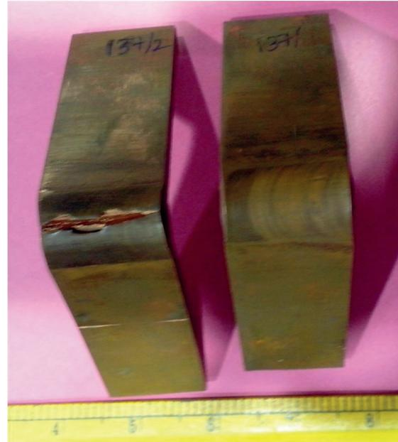
**Fig. 8** - Bend tested specimen
