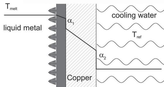
**Fig. 3** - Schematic heat transport from the melt to the cooling water
