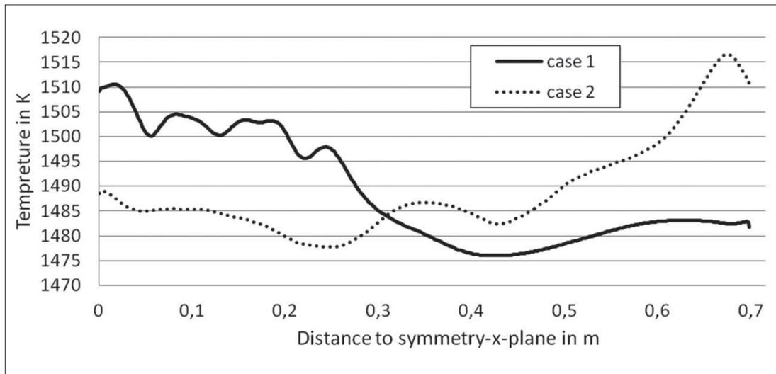
**Fig. 6** - Temperature distribution at the contact-line of solidified strip and casting roll at the casting gap for case 1 and 2
