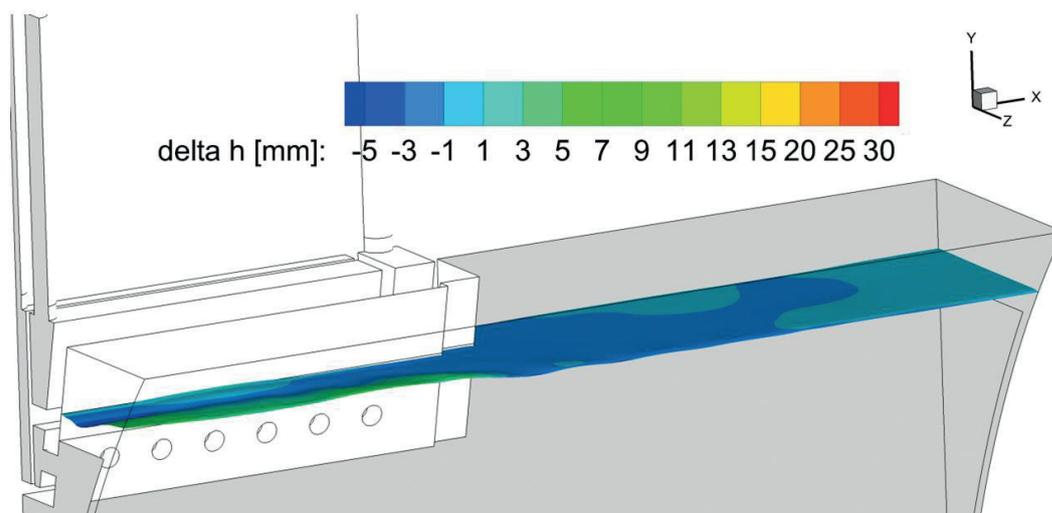
**Fig. 7** - VoF Simulation of the free surface for case 1
