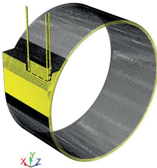
Fig. 2 - Quarter Mesh of the twin roll strip caster
