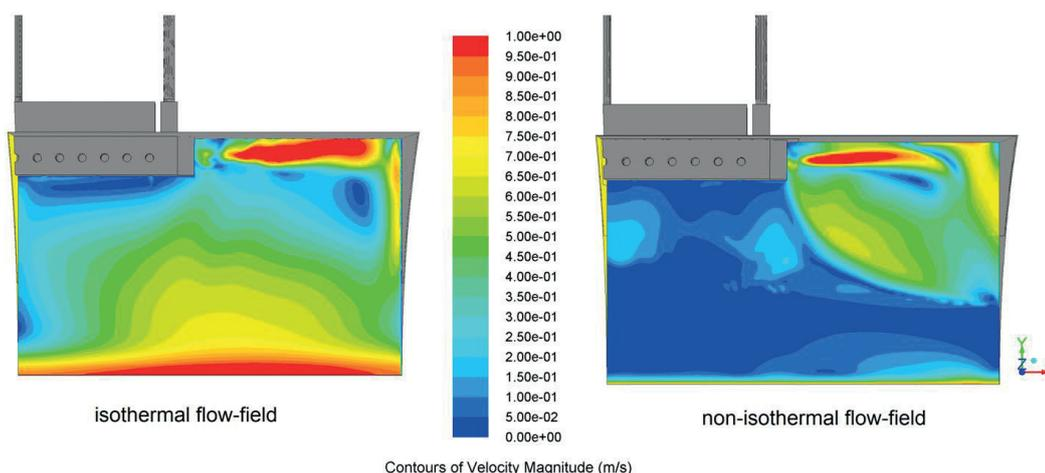
**Fig. 4** - Comparison of isothermal and non-isothermal flow for flow-case 2
