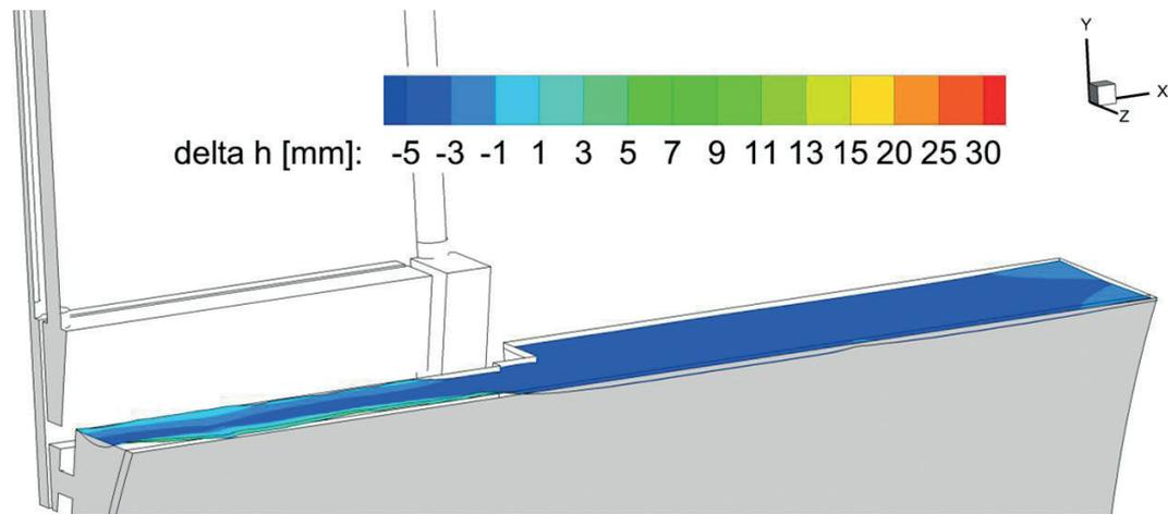
**Fig. 8** - Free surface for case 1 calculated from the pressure distribution
