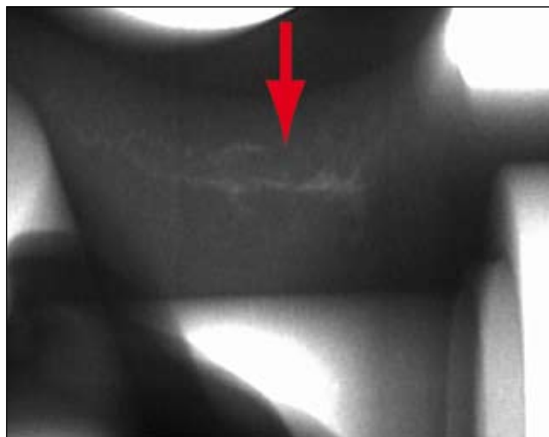
Fig. 2 - X-ray image of one end of the casting. The arrow indicates the presence of macroporosity.
