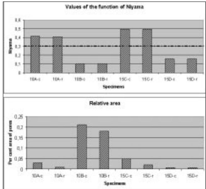
Fig. 7 – Value of the function of Niyama (upper); relative area of the pores in the specimens (lower).
