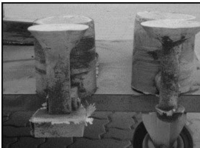
Fig. 6 – The two types of gating system: rectangular (left) and circular (right).
