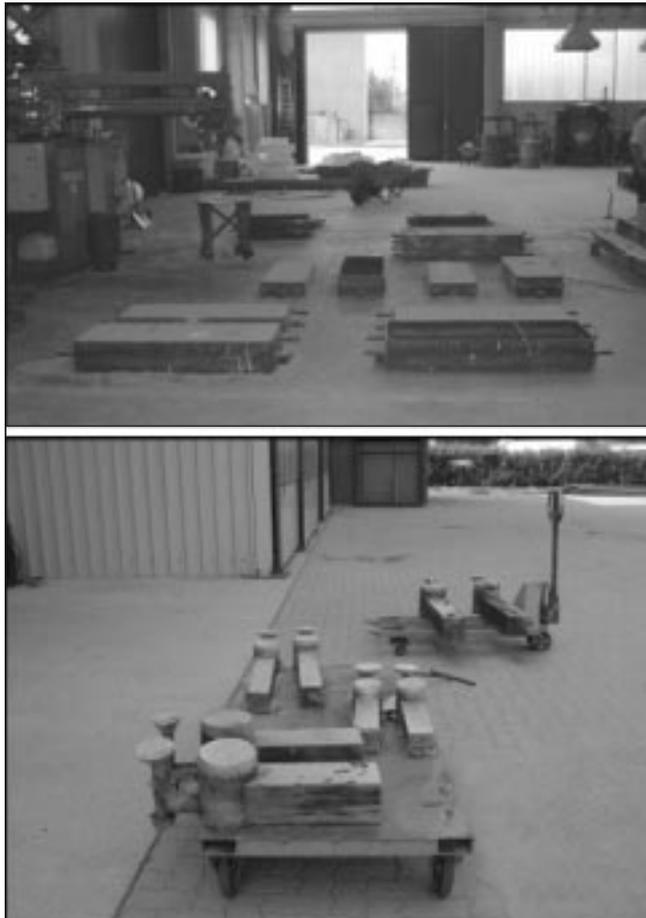
Fig. 5 – The moulds (upper), the eight specimens (lower).
