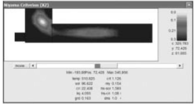
Fig. 3 - Visualization of the result through 2D image of the criterion of Niyama for the specimen 15D-c.
